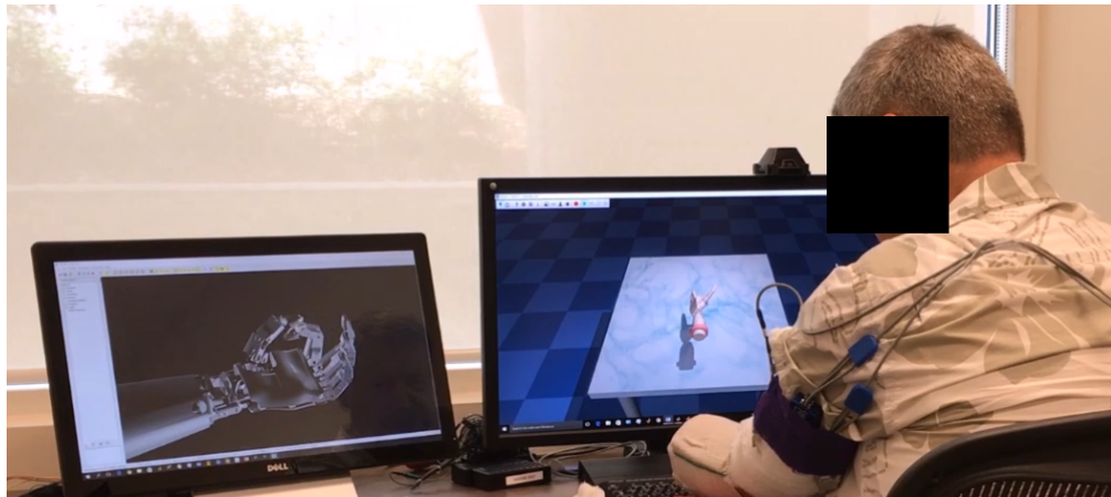
Figure 3.1: Experimental setup used in this work. The study volunteer (HS2) had intramuscular EMG electrodes implanted in his arm and was asked to follow the the movements shown on the screen using his phantom limb. The screen on the left was used to show the movements during the training phase. The screen on the right showed the decoder results during a possible online phase. ©2019 IEEE [27].
