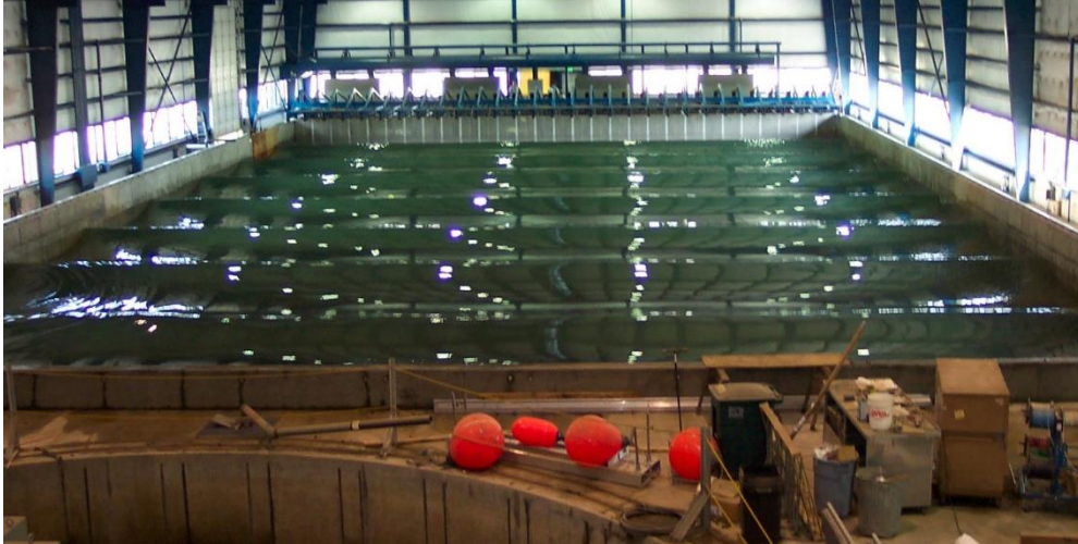
Figure 3.9: Regular, shore normal waves generated in the DWB at Oregon State.
