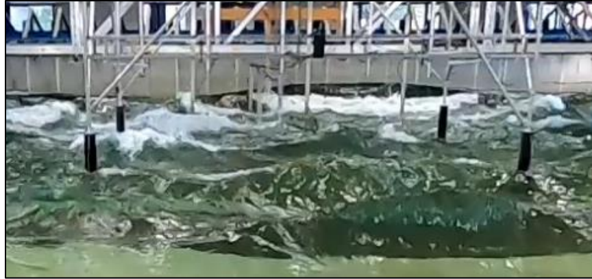
Figure 6.11: GoPro ® snapshot of waves under the instrumentation frame taken from basin beach during the bidirectional regular wave case.
