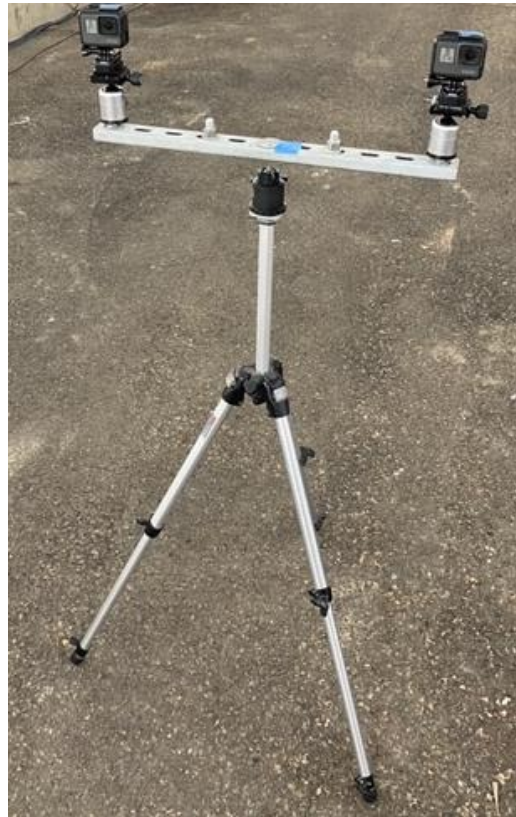
Figure 3.3: A pair of GoPros® (Pair 1) with their Unistrut mount attached to a movable tripod for preliminary testing.
