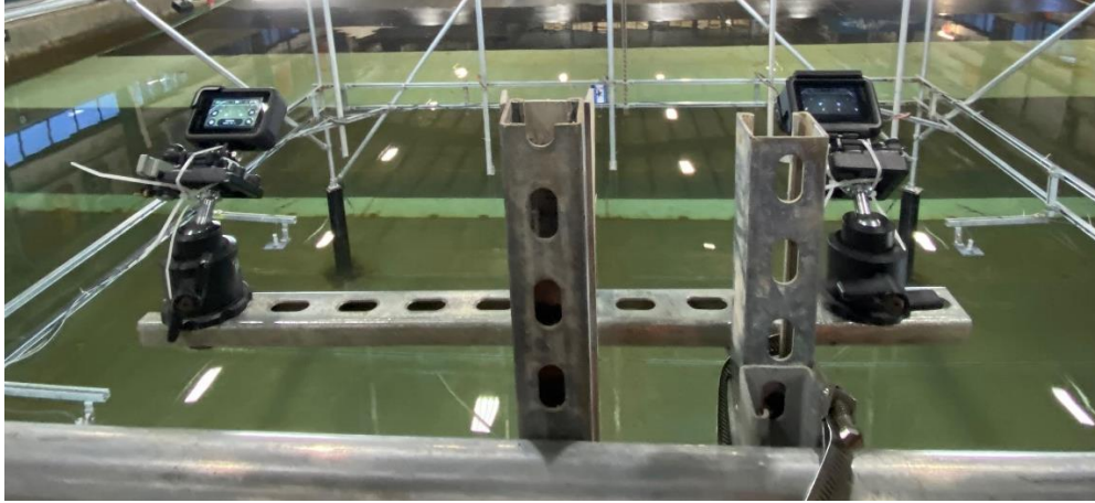
Figure 3.4: GoPro® stereo pair mounted to instrumentation frame.
