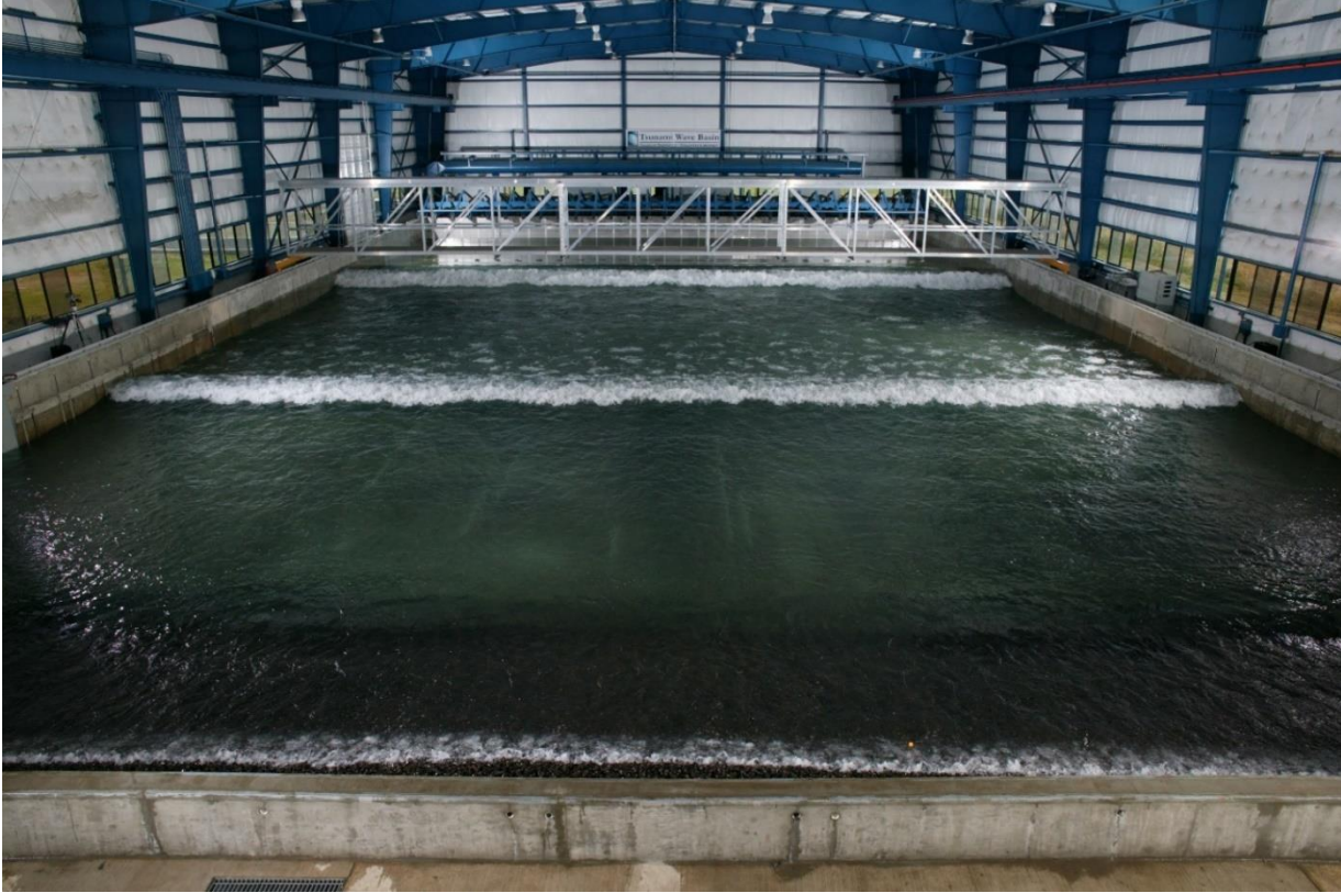
Figure 3.1: Image of the DWB generating breaking long-crested waves looking toward the wave-maker.
