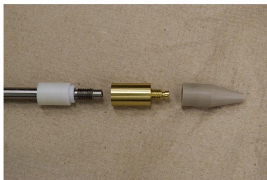
Figure 4. (top) Custom electrode head (Pt disc, r = 50\mu\text{m} ) attached to a Pine Research rotator shaft. Tip is 4.5 mm in diameter, tapering to 12 mm at the white sleeve shown. (middle, bottom) Attachment of custom tip to commercial rotator shaft.
