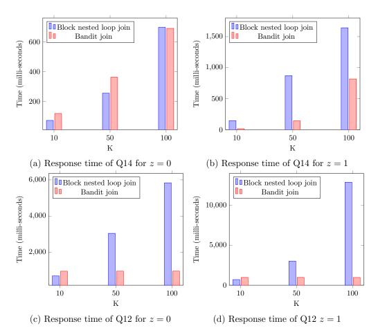
Figure 4.2: Response time of bandit join compared to block nested loop join for different values of k
