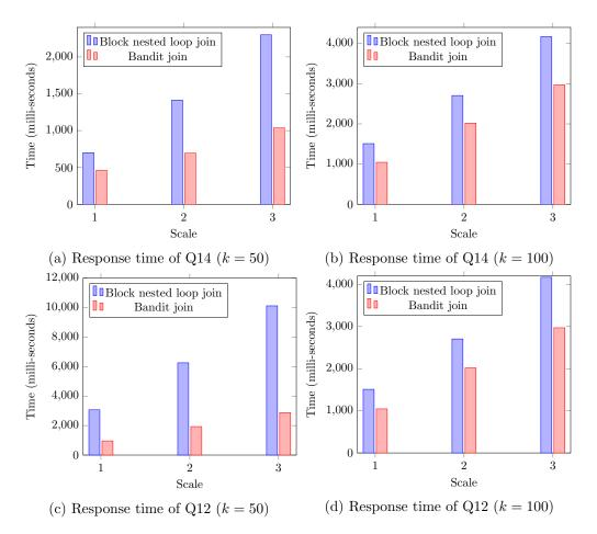
Figure 4.5: Impact of database size on the response time of bandit join and block nested loop join
