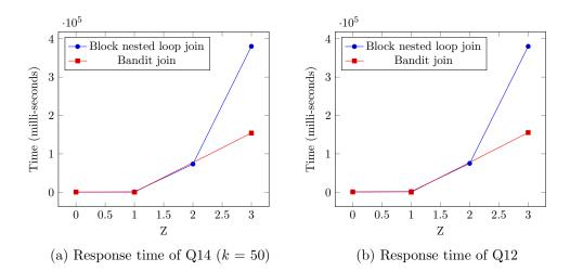
Figure 4.7: Impact of data skew on the response time of bandit join and block nested loop join (k = 100)
