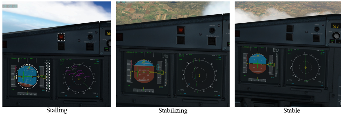
Figure 3.12: Primary Flight Display (PFD) during the stall, stabilization, and stable stages of X-plane flight simulation for the first scenario
