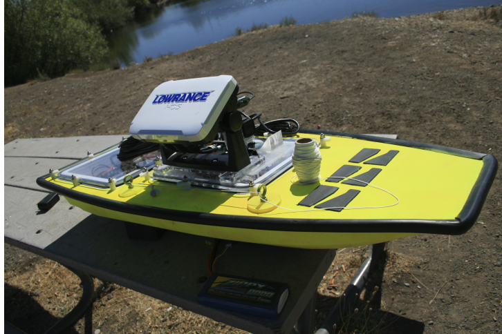
Figure 6.11: Platypus Lutra Autonomous Boat with Lowrance depth sonar used in field trial experiments [3]
