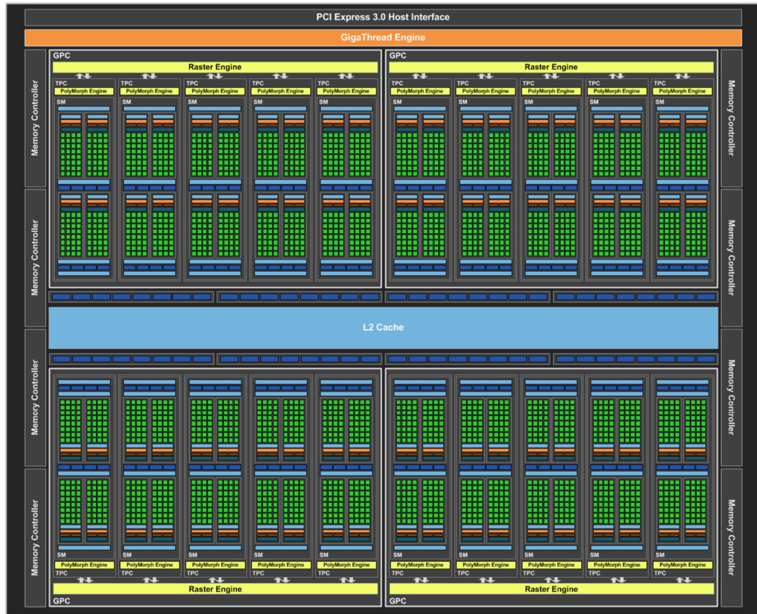
Figure 1.1: GPU Diagram (Pascal Architecture).
