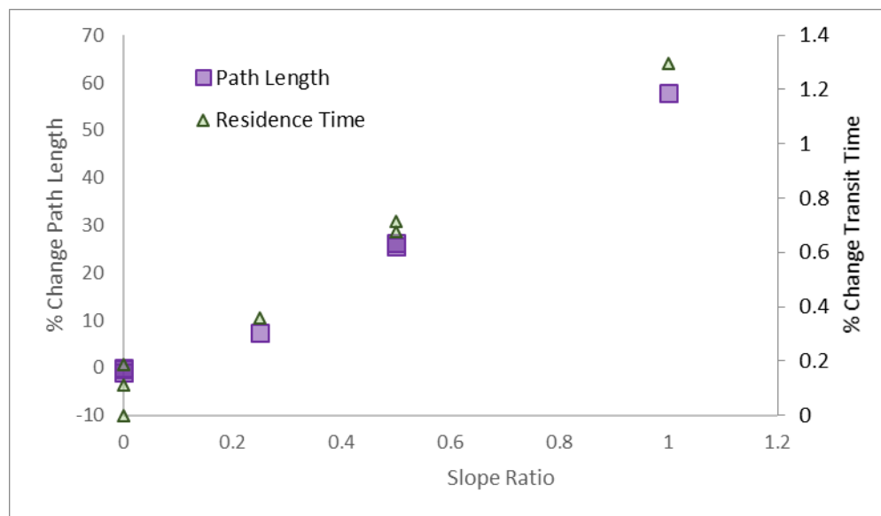
Figure 19. Percent change in path length (orange circles) and transit time (blue diamonds) compared to the initial ratio of slopes defined as \tan(\gamma)/\tan(\beta) for Models 1-7. For models with a zero stream slope or hillslope, the path length decreases slightly as the water table lowers. For the four models 3D models, lowering the water table changes the driving gradients for flow, increasing the path length and transit time.
