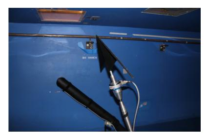
Figure 3.8: The Oregon State University closed loop wind tunnel with stunt kite test geometry.
