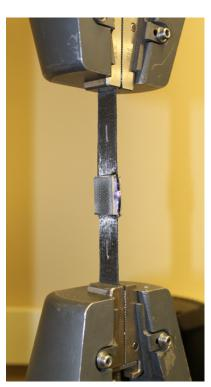
Figure 4.11:Double lap joint sample mounted in the Instron
