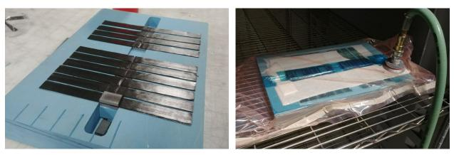
Figure 4.10: Manufacturing process using a Renshape mold to layup on and vacuum bag to get compaction of the prepreg material.
