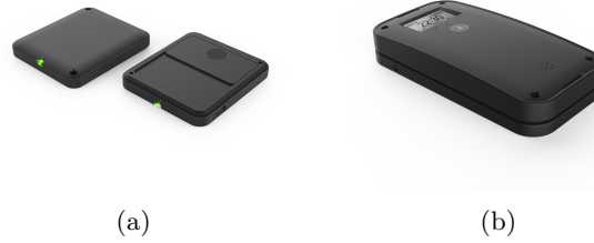
Figure 4.6: The conceptual designs for (a) field-deployable SS tags and (b) a unified GW server device. LCD: liquid crystal display.
