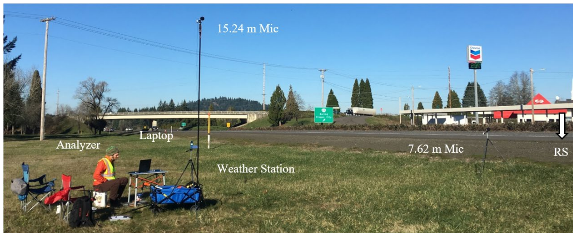
Figure 2.3 Exterior sound measurement setup
