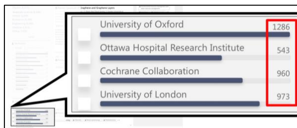
Figure 7 Facets Drive Fixes Practice. The filtering widget originally included a counts column (right). The team decided that task-motivated users like Abi might not see it as a filtering device, since it looks more like statistics. Team O removed it.
