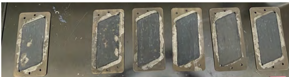
Figure 4.17: The final catalyst coating of the bottom surface of the coolant channel (which makes up the top half of the reaction channel).
