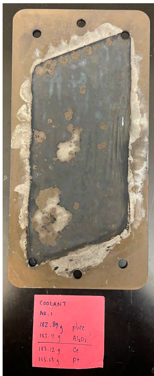
Figure A.7: Coolant plate 1 and corresponding weights measured after drying and calcination for each step of the catalyst coating process.
