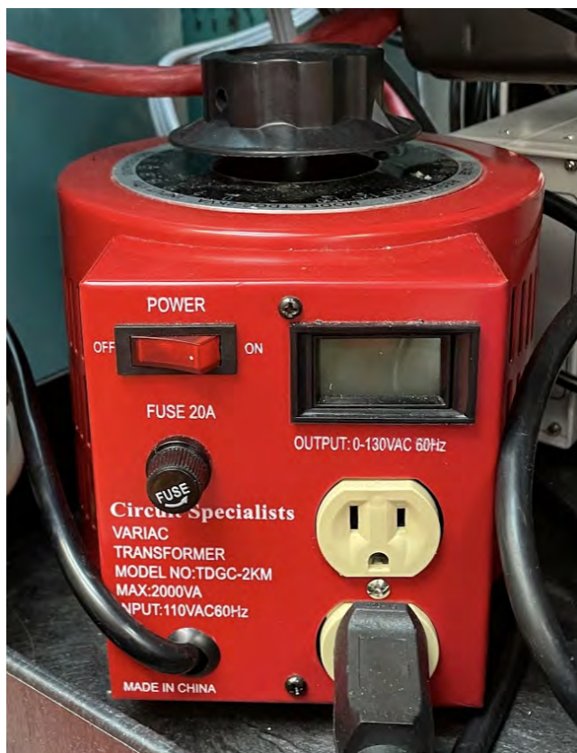
Figure 5.17: A Variac TDGC-2KM transformer.
