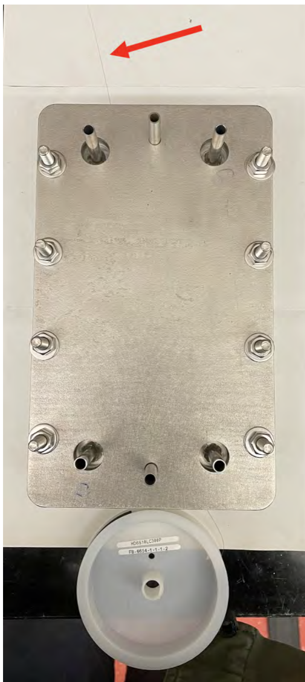
Figure 3.24: A top view of the reactor assembled after compression of gaskets. The arrow points to the LUNA fiber integrated into the reactor via instrumentation plate.
