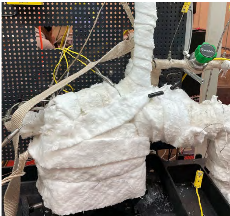
Figure 5.28: The reactor wrapped in the white Cerablanket sheet insulation.
