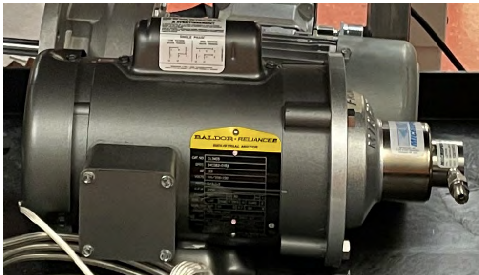
Figure 5.16: The Baldor motor and Micropump GA-V23 pump head assembly.
