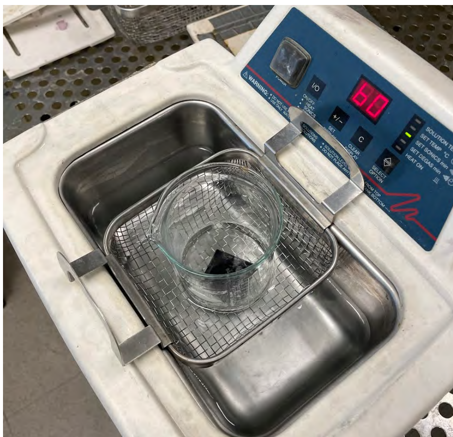
Figure 4.21: The ultrasonic adhesion test setup.
