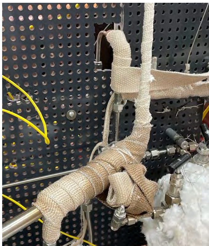
Figure 5.27: The gas cartridge HX wrapped in a base layer of the silica strip insulation.
