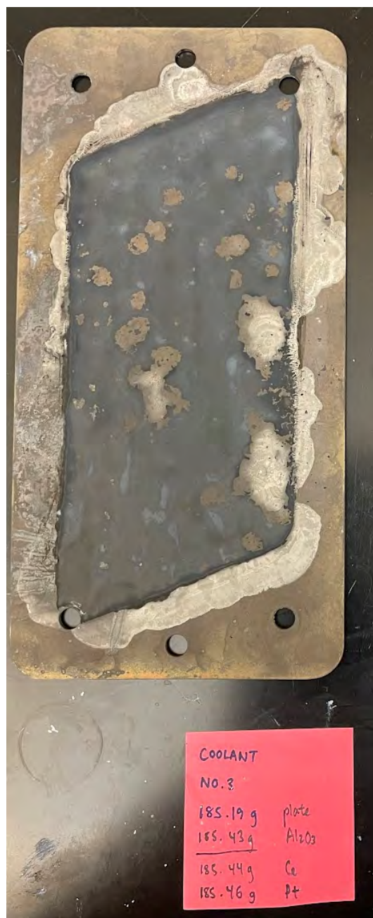
Figure A.8: Coolant plate 2 and corresponding weights measured after drying and calcination for each step of the catalyst coating process.
