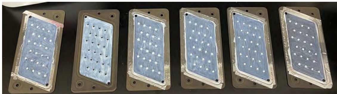
Figure 4.14: Masked reactant channels coated with the alumina slurry. The mask was removed on the second plate.
