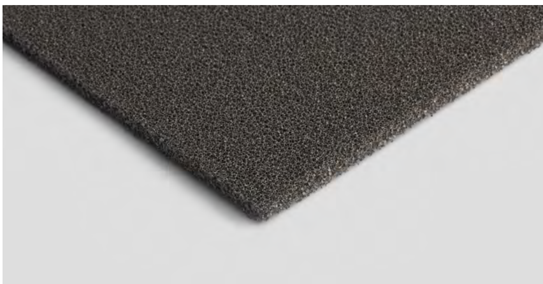
Figure 2.7: Fecralloy®, a popular metal foam support material, shown in sheet form [40].
