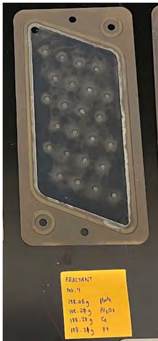
Figure A.4: Reactant plate 4 and corresponding weights measured after drying and calcination for each step of the catalyst coating process.
