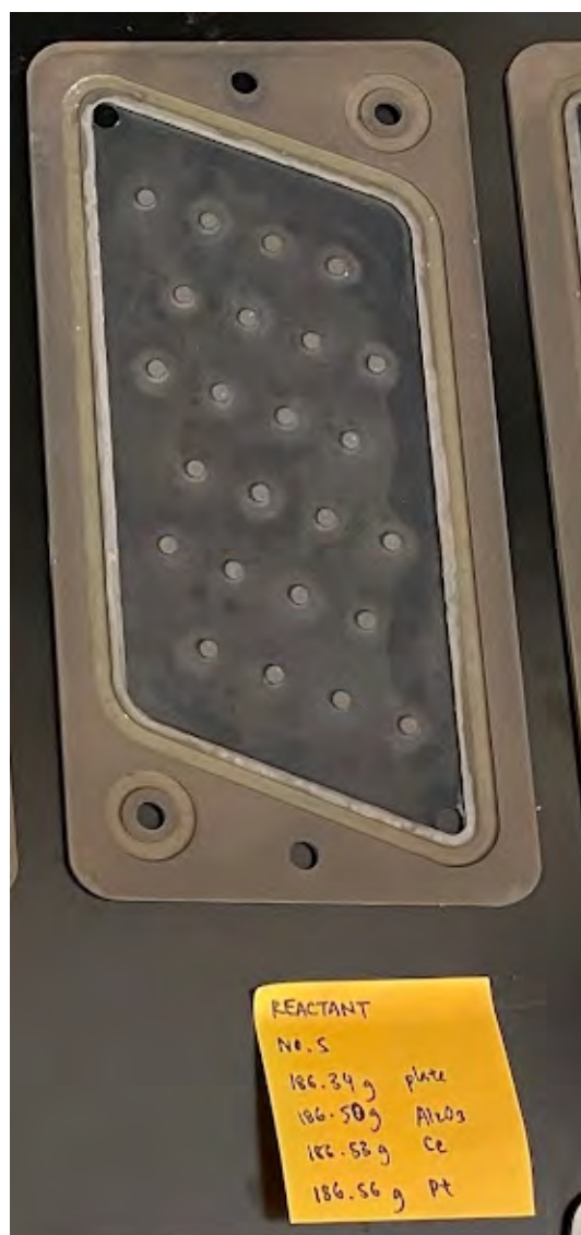
Figure A.5: Reactant plate 5 and corresponding weights measured after drying and calcination for each step of the catalyst coating process.
