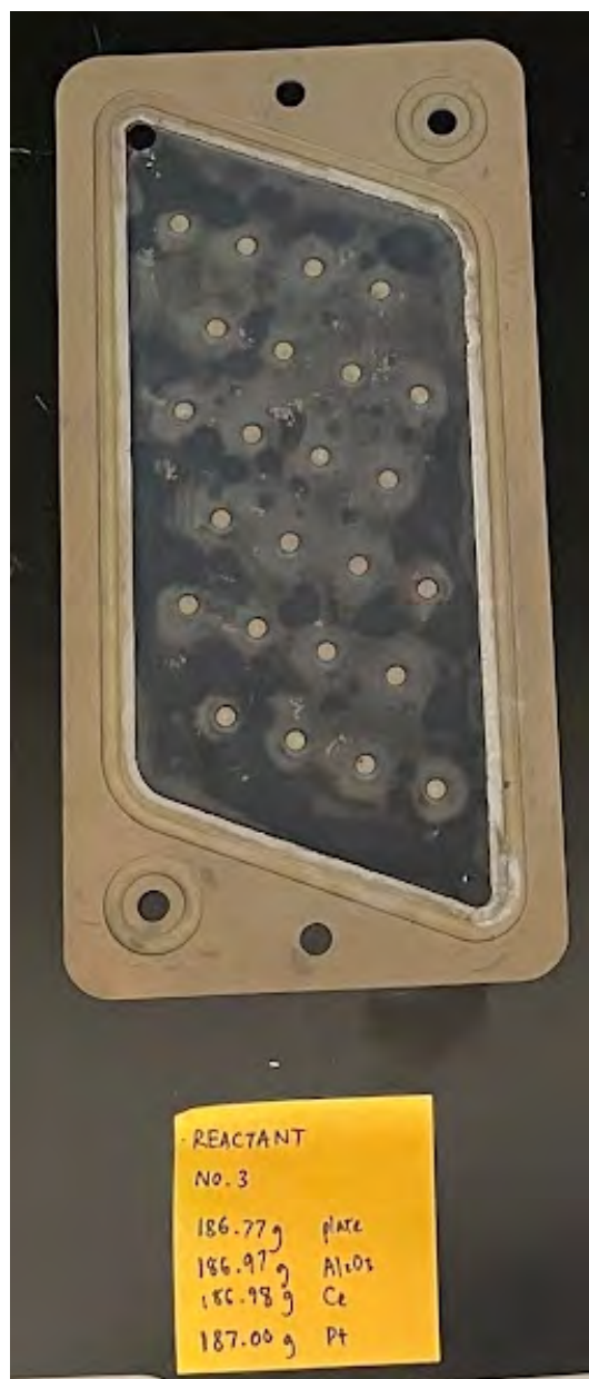
Figure A.3: Reactant plate 3 and corresponding weights measured after drying and calcination for each step of the catalyst coating process.
