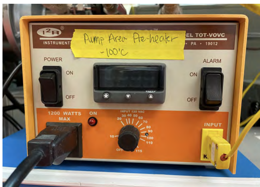
Figure 5.19: A PID temperature controller.
