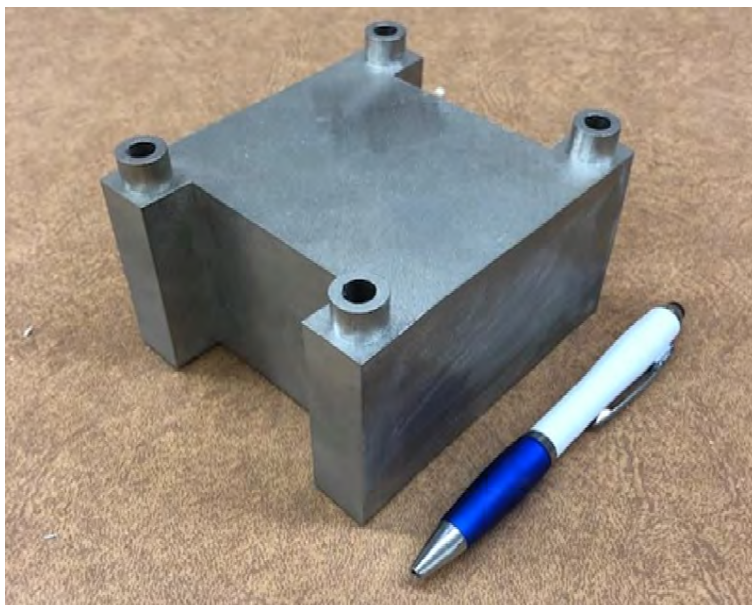
Figure 2.20: Additively manufactured monolithic reactor (pen for scale) developed by Tolley [43].
