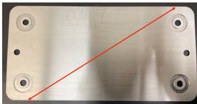
Figure 3.18: An image depicting the predicted milling path for the fiber channel.
