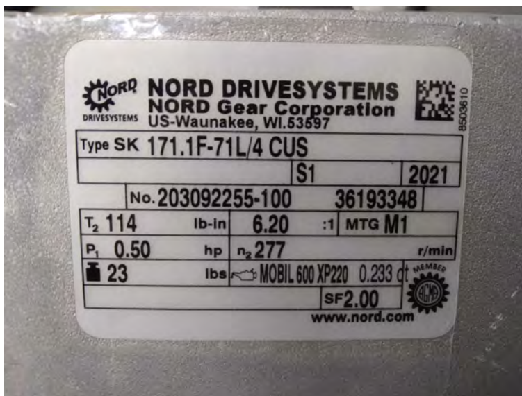
Figure 5.13: Nord gearbox nameplate.
