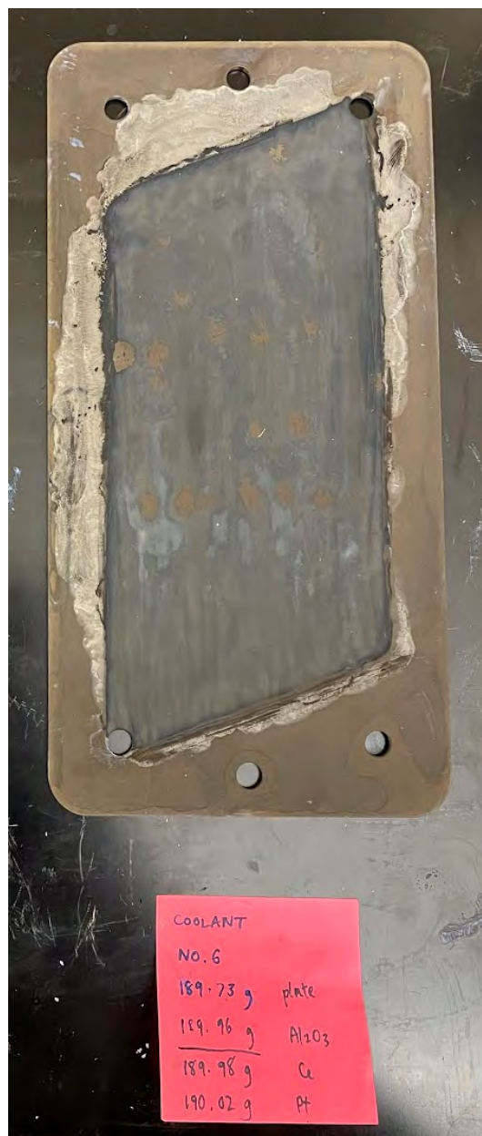
Figure A.11: Coolant plate 6 and corresponding weights measured after drying and calcination for each step of the catalyst coating process.
