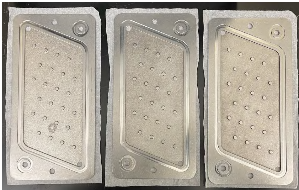
Figure 4.9: Three of the six reactant plates laid out after being cleaned with acetone.
