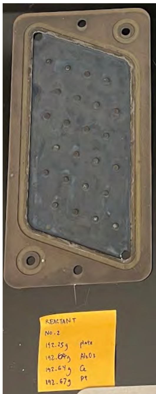
Figure A.2: Reactant plate 2 and corresponding weights measured after drying and calcination for each step of the catalyst coating process.
