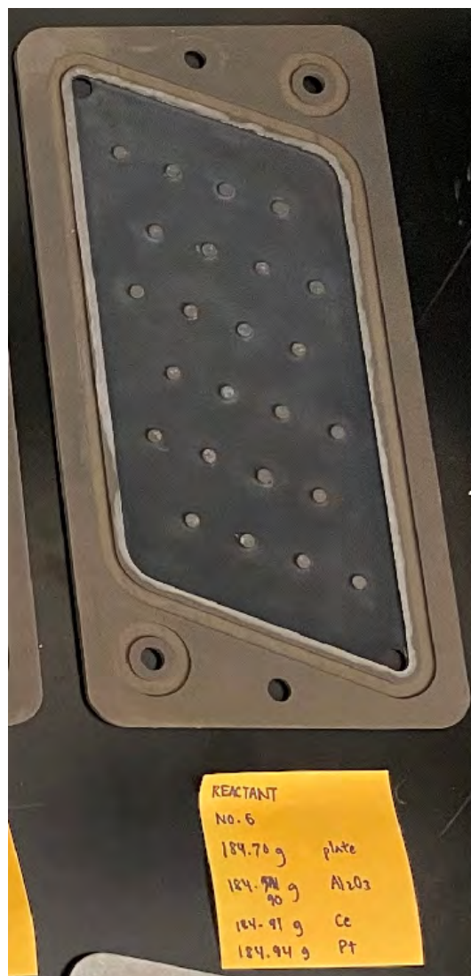
Figure A.6: Reactant plate 6 and corresponding weights measured after drying and calcination for each step of the catalyst coating process.
