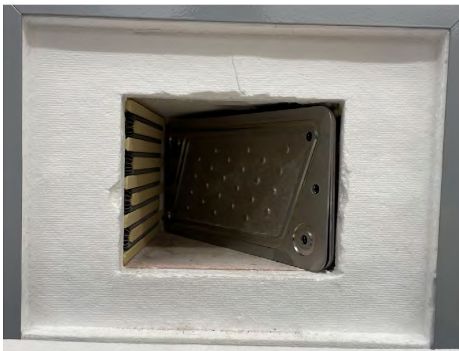
Figure 4.10: Three of the six reactant plates arranged in the Thermolyne furnace before thermal pretreatment.
