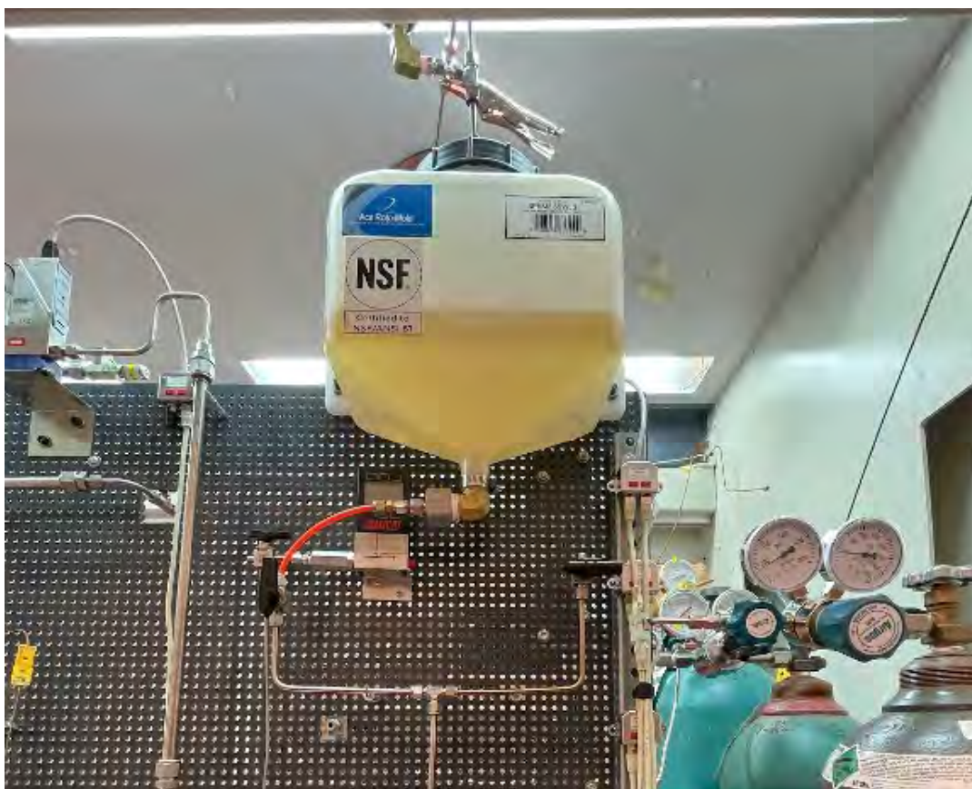
Figure 5.4: The liquid loop is vacuum filled from a reservoir of Therminol 72.
