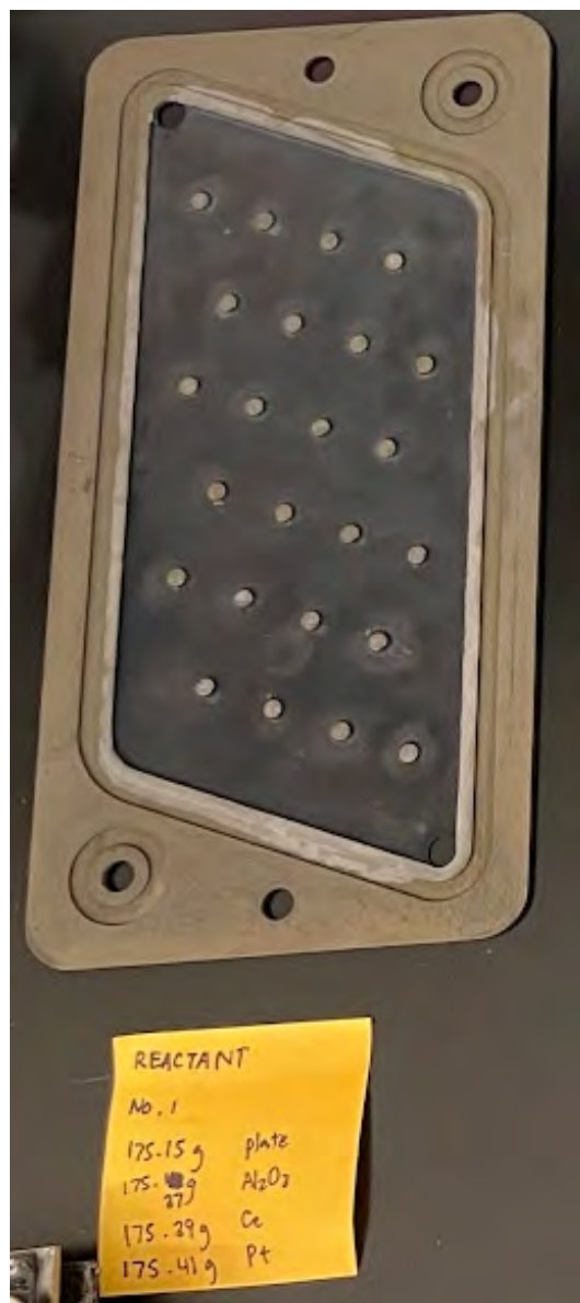
Figure A.1: Reactant plate 1 and corresponding weights measured after drying and calcination for each step of the catalyst coating process.
