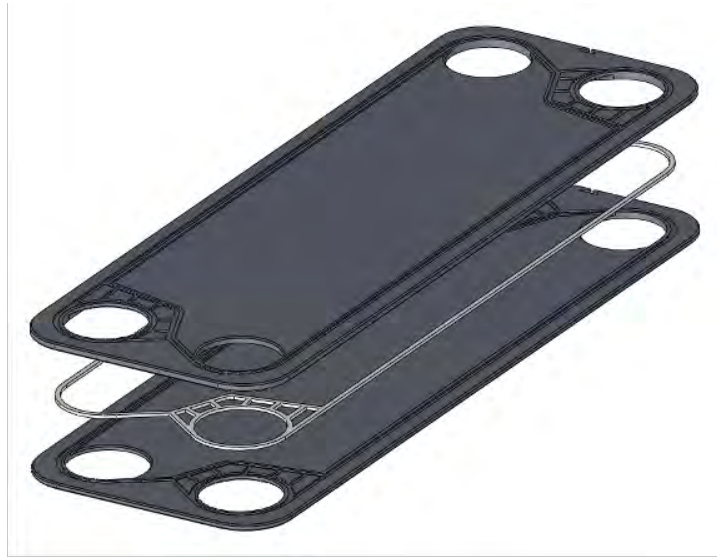
Figure 3.2: The first design iteration focused only on the design of the unit cell, which consists of a reactant plate, gasket, and coolant plate.
