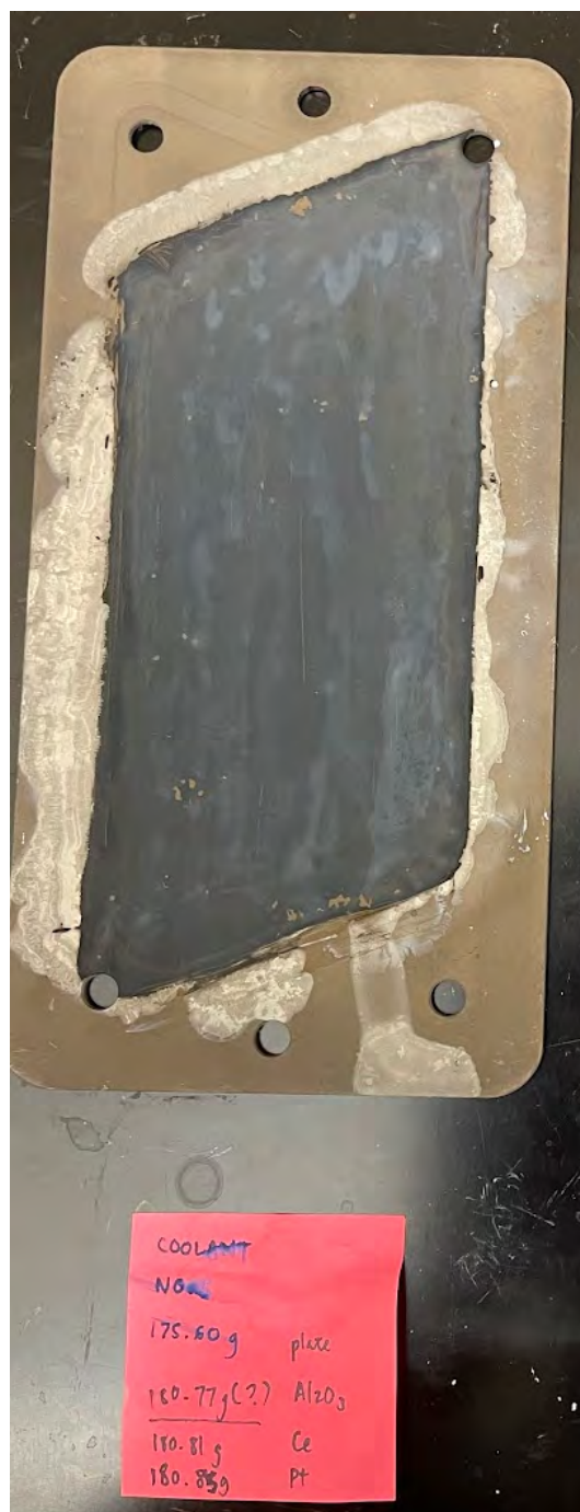
Figure A.10: Coolant plate 5 and corresponding weights measured after drying and calcination for each step of the catalyst coating process.
