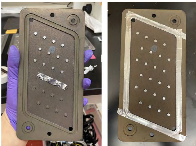
Figure 4.13: An aluminum tape mask was applied to the reactant plates to shield mating surfaces from being coated in catalyst.
