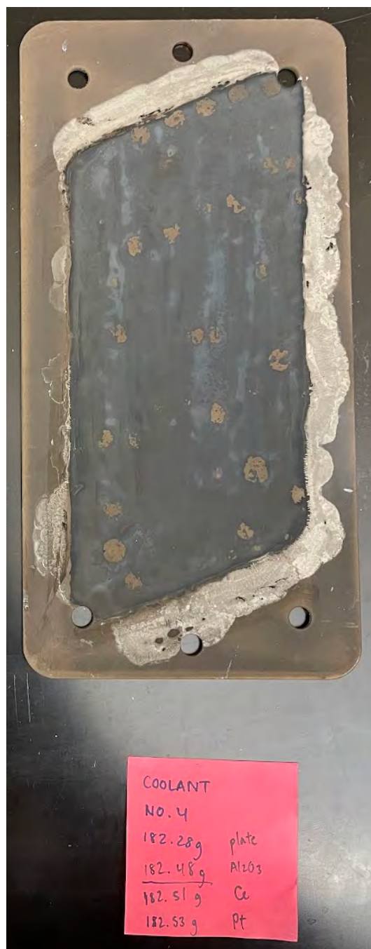
Figure A.9: Coolant plate 3 and corresponding weights measured after drying and calcination for each step of the catalyst coating process.
