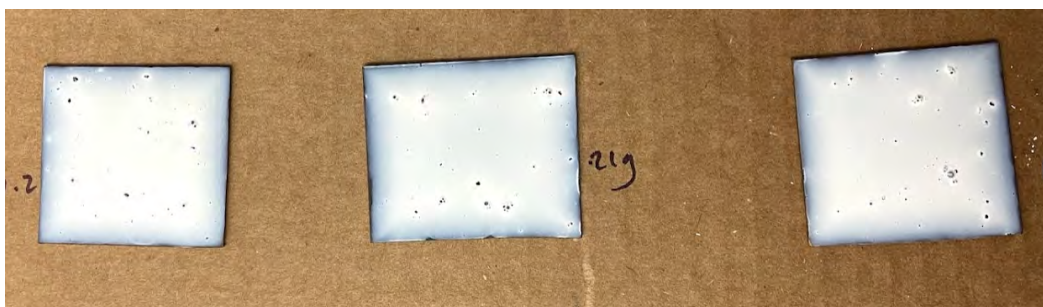
Figure 4.6: Three coupons after drying of the initial alumina washcoat layer. The disruptions to the white washcoat are pieces of PVA that were unincorporated during the mixing of the binder in DI water because the mixing temperature was too low. The final recipe corrected this by increasing the mixing temperature to 120°C.
