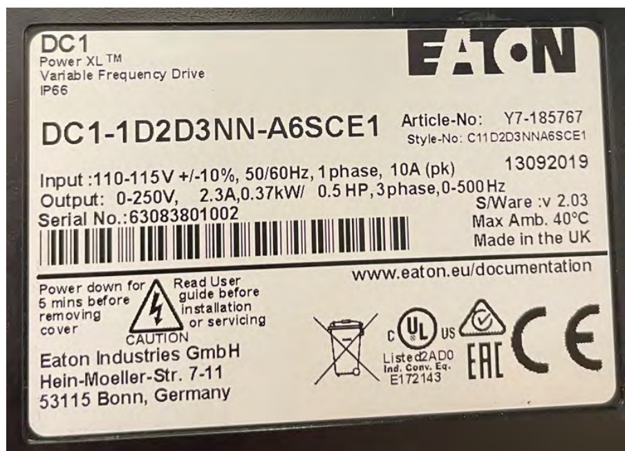
Figure 5.12: Eaton VFD nameplate.
