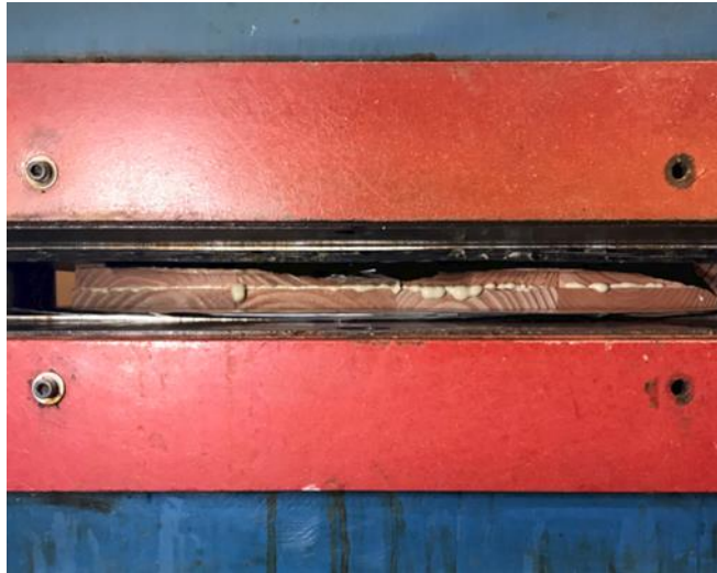
Figure 3-2, PU compression block assembly in cold press
