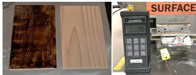
Figure 3-3, PF sample preparation; single bondline (left) and hot-pressing in 6-inch by 6-inch electrically-heated press (right)
