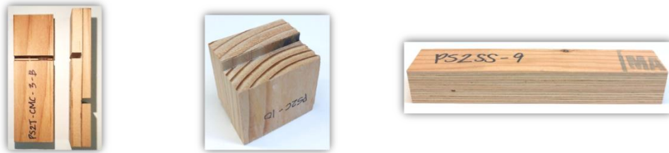
Figure 3-4, Completed lap-shear in tension specimen (left), lap-shear in compression specimen (center) and short-span shear in bending specimen (right).
