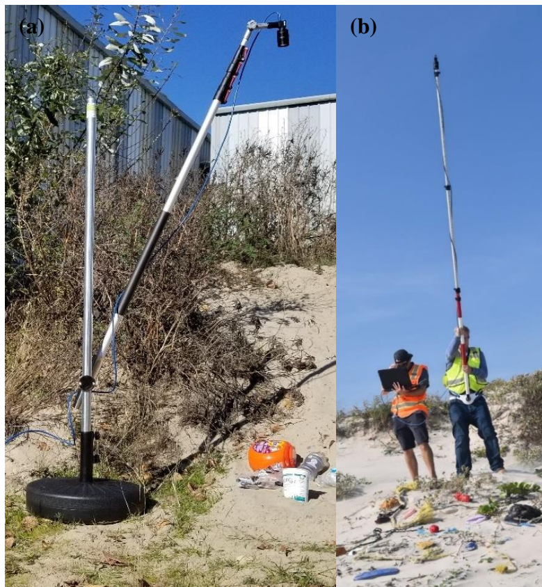
Figure 3. (a-b) Camera configurations used in fieldwork scenarios. (a) fixed setup used at O.H. Hinsdale Wave Research Lab (left); (b) mobile setup used in Corpus Christi TX (right).
