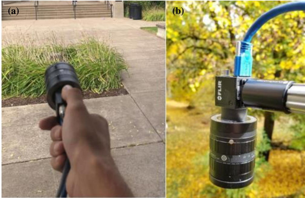
Figure 2. (a-b) FLIR Blackfly S and Fujinon 12.5-mm focal length lens. (a) Camera and lens held in hand; (b) Camera and lens attached to pole.
