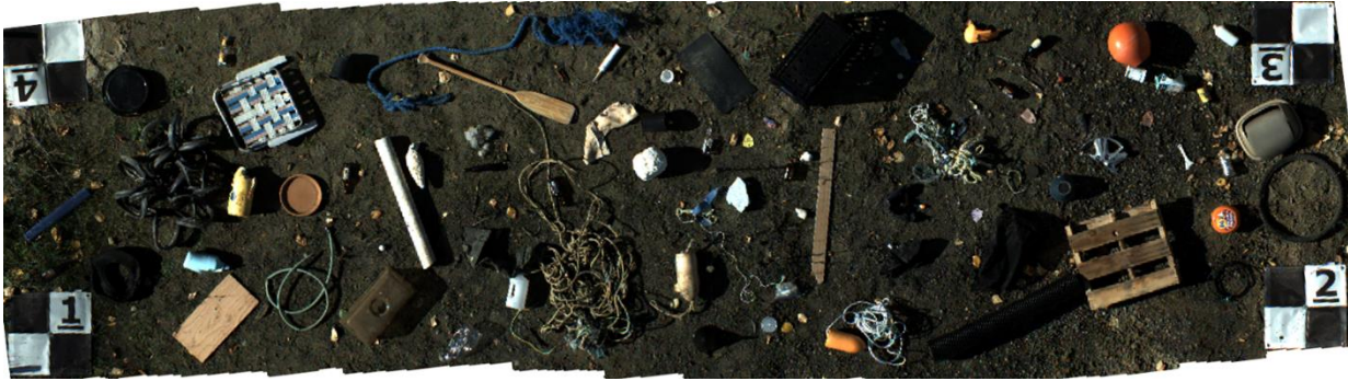
Figure 19. Wavelab debris field, used for evaluating band correlations and debris classification. 3.6m AGL sensor height, 34 images total.
