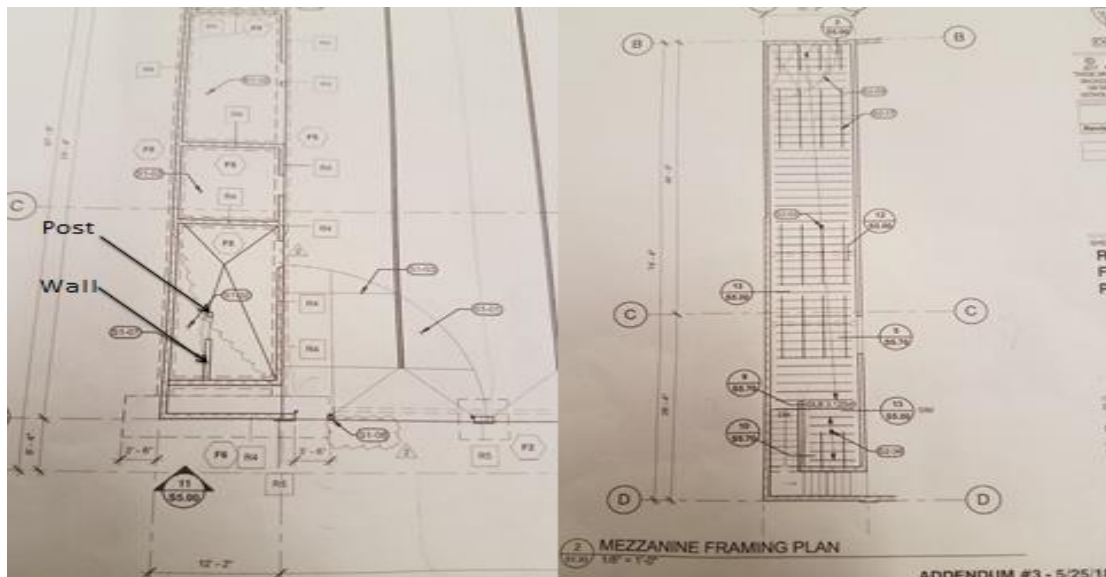
Figure 2-4. Mezzanine framing plan (right image) partially supported by the post and wall (left image).
