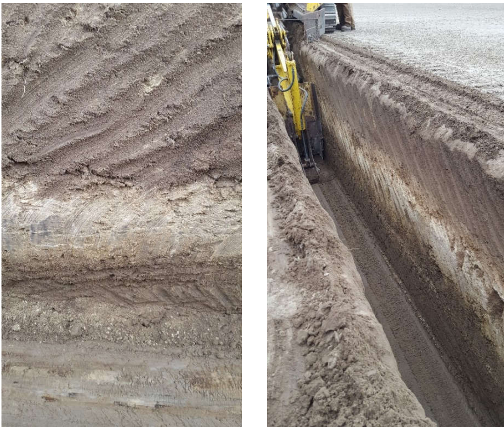
Image 3. Potato site at Klamath Basin Research and Extension Center. This trench, dug across the potato site, is in map unit 19A with 72% Fordney Series. Soil demonstrated a strongly-cemented silica layer not described in the Fordney series description. Potatoes are shallow rooted and likely would not have been influenced by this horizon.
