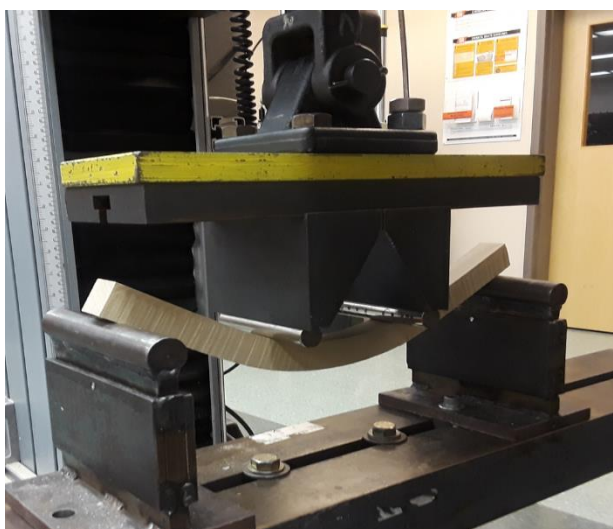
Figure 24 - Photo showing extreme deflection of a small clear beam from rail tie 1600 compared to all other beams.
