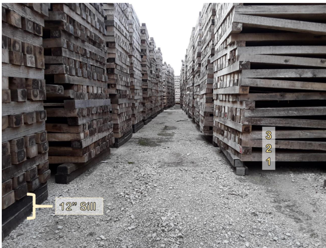
Figure 3 - Air seasoning rail ties in German Stack configuration. Sampled courses (tiers) are labeled 1, 2, 3; and conventional 12" sill height is indicated. Reduced sill heights were arranged by using a single treated rail tie footing, where two are shown here.
