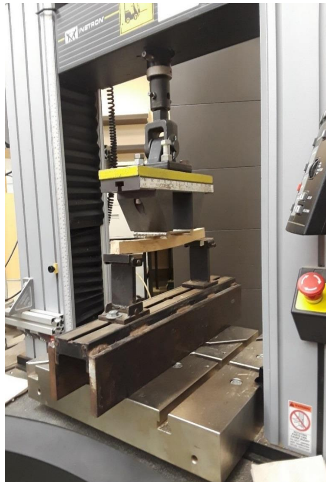
Figure 6 - A small clear beam under 4-point loading with Instron Universal Testing Machine.
