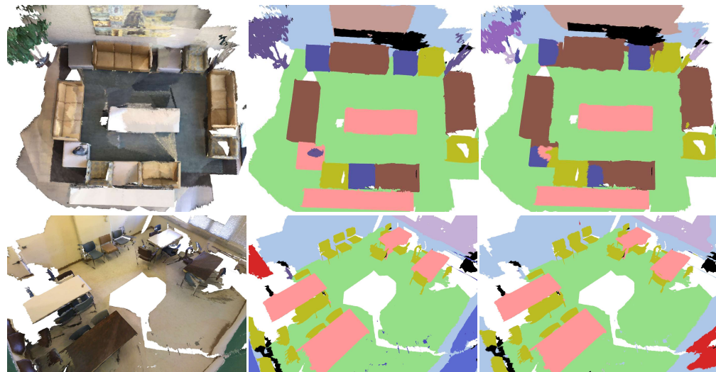
Figure 2.14: Examples of semantic scene labeling. The images from left to right are the input scenes, the ground truth segmentation, and the prediction from PointConv. For better visualization, the point clouds are converted into mesh format. Best viewed in color.
