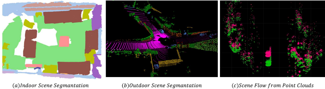
Figure 4.2: Applications of PointConvFormer. PointConvFormer can serve as the backbone for various 3D scene understanding tasks, such as semantic segmentation for indoor/outdoor scenes, and scene flow estimation from point clouds
