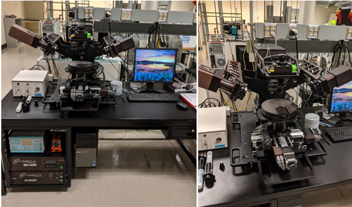
Figure 5: The M-2000X spectroscopic ellipsometry system used in these results (pictures taken by author). The polarizer and analyzer arms (left and right, respectively) are pointed down at the sample stage in the center.
