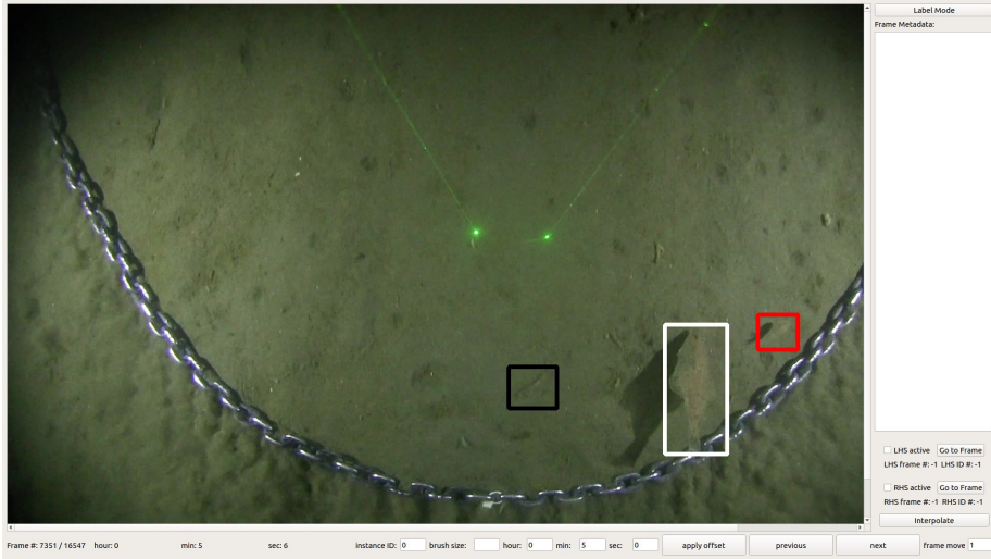
Figure 3: Screenshot of the Fishlabeler UI with three fish detections annotated. The different colored bounding boxes correspond to different instance IDs. The bounding boxes should cover the entirety of the fish, but be as tight as possible to the fish (i.e. not have extraneous non-fish background pixels with in the bounding box).
