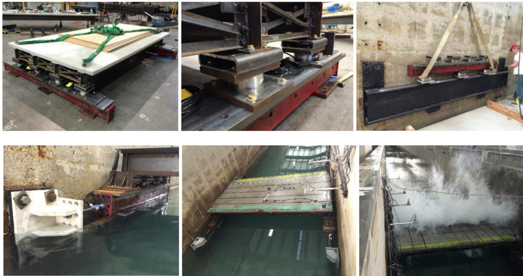
Figure 3. Test specimen and components during the pre-test assembly in the Large-Scale Structures Laboratory at the University of Nevada, Reno (UNR) and during the hydrodynamic testing phase in the LWF at Oregon State University.
