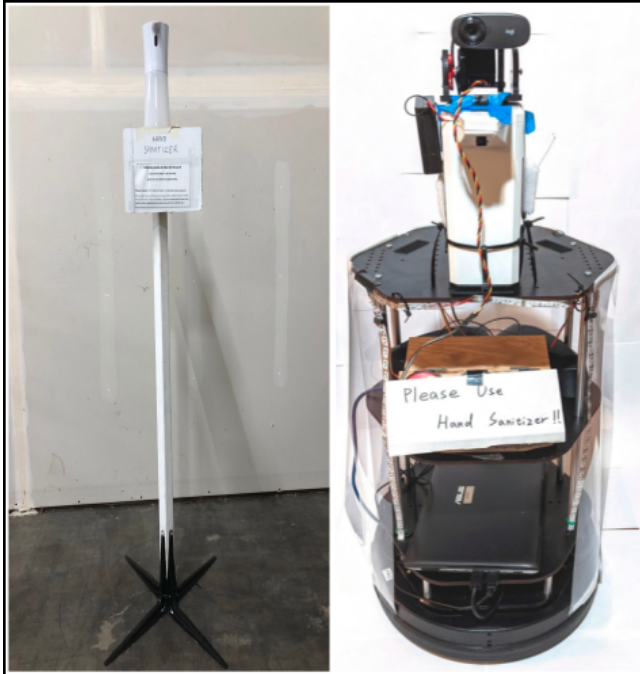
Figure 2. Hardware design of Stick (on left) and SanitizerBot (on right)
