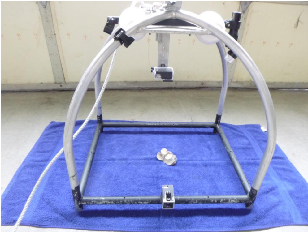
Figure 11. Benthic Lander set-up used to capture underwater photos in the subtidal survey. Aluminum frame provides a platform for a GoPro camera and for oblique illumination by a battery-operated, LED dive light. Surface area of the image frame is 0.5 m 2 . A pair of plastic net floats provided buoyancy at the top of the lander and served to maintain the proper orientation during descent to the bottom.
