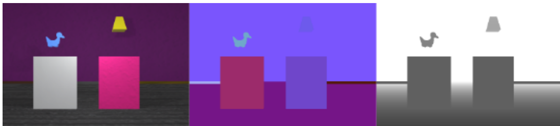
Fig. 2. An example of input passed to the system where the left image corresponds to an RGB frame, the middle image corresponds to a ground-truth segmentation mask and the right image to a depth image.
