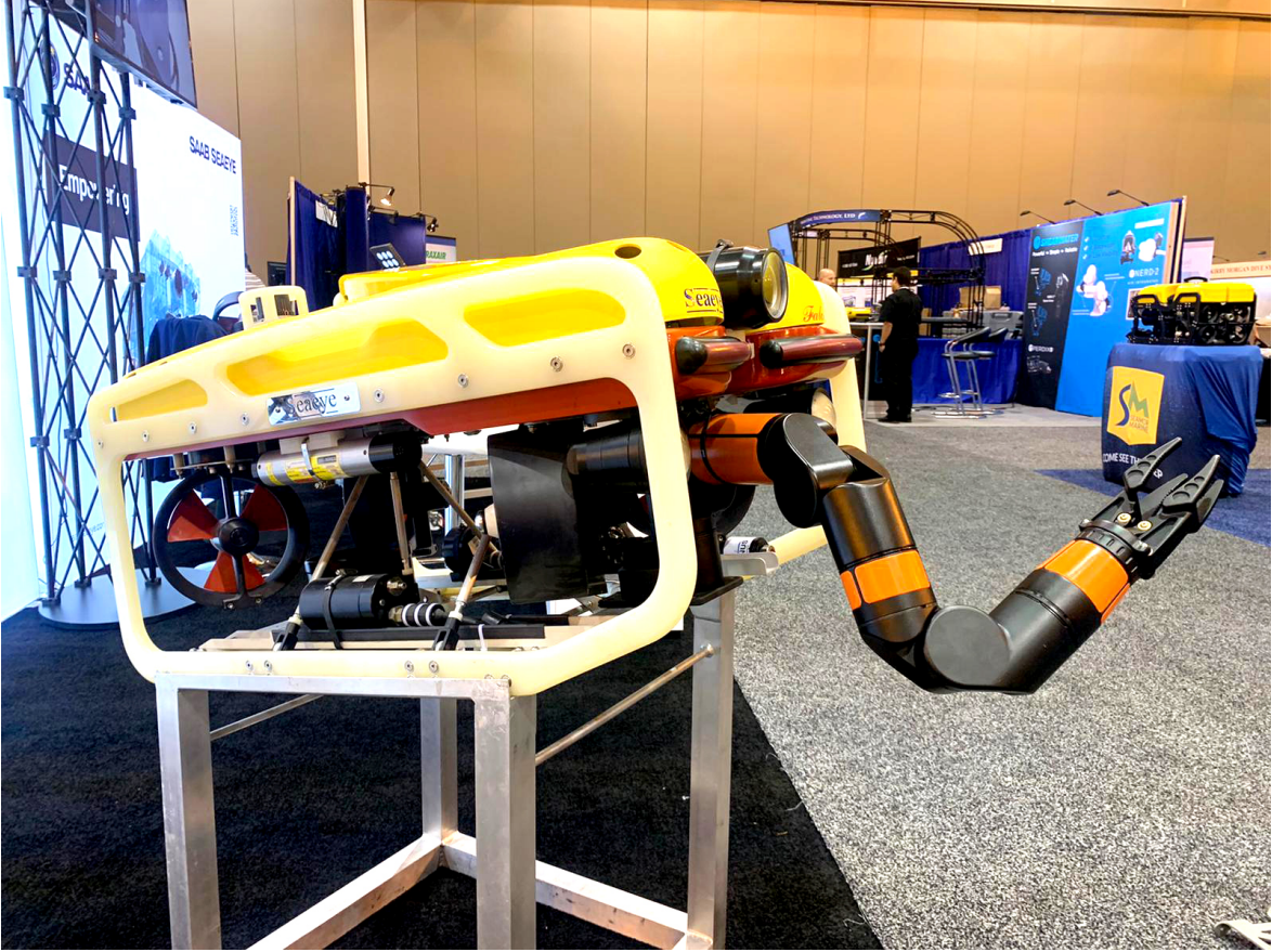
Figure 3: Picture of sample vehicle for underwater manipulation
