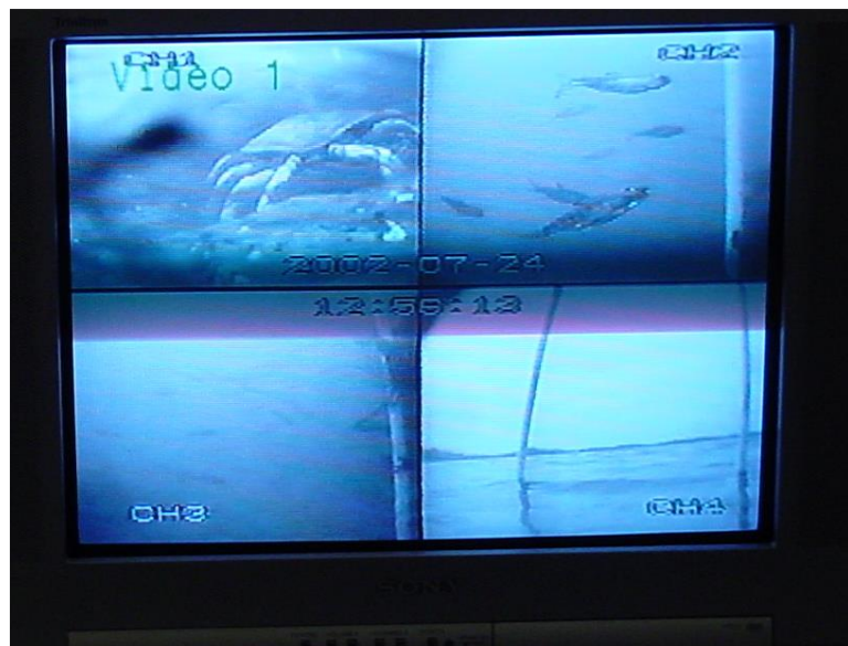
Figure 6.3. Example sampling data gathered using videography. The four views represent different cameras located at different elevations off the channel bed within the same sampling station (pole).
