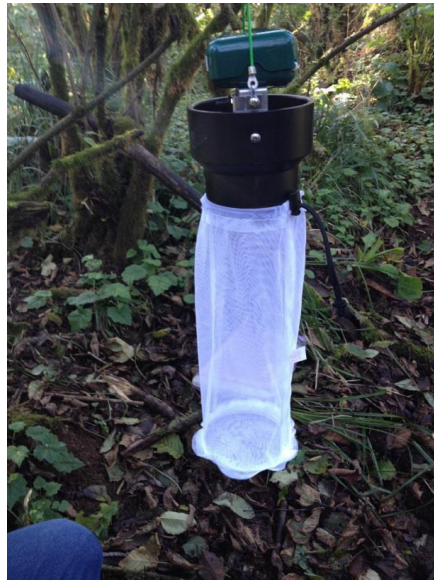
Figure 8.5. CDC trap hung from a tree limb during trapping to collect adult mosquitoes at the SFC site.
