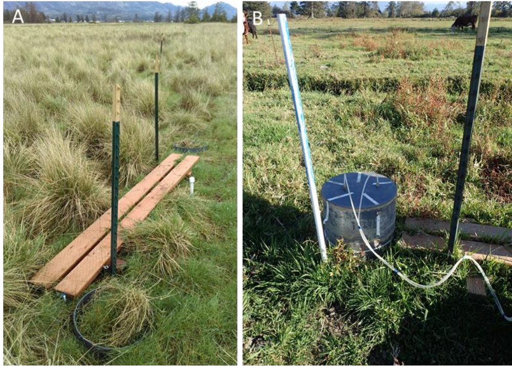
Figure 9.2. Field measurements of greenhouse gas emissions: (A) boardwalk, two chamber bases, and small groundwater well installed in high marsh at Dry Stocking Island, and (B) chamber top placement on one of the chamber bases at a disturbed agricultural site. Photos by C. Janousek.
