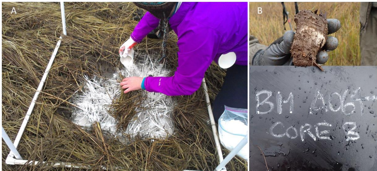
Figure 2.3. (A) Establishment of a feldspar marker horizon layer inside a 1.0 m 2 plot in 2013, and (B) example of a sediment wedge collected in 2018 to measure accretion 4.9 years after plot establishment. Photos by C. Janousek.
