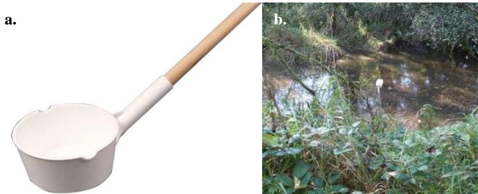
Figure 8.4. (a) Mosquito dipper used for larval sampling. (b) Mosquito dipper standing upright in vegetation at one of the SFC sampling stations.
