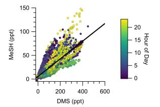
**Figure 3.** Correlation of DMS and MeSH mixing ratios at a 2 min averaging time colored by hour of day of the observation. Hour of day is in local time (UTC – 7). The linear least squares best fit is plotted as the solid black line. The slope of the best fit line is 0.19, and  $R^2 = 0.61$ .
