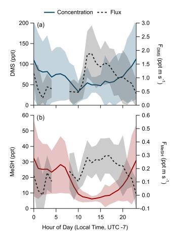
**Figure 4.** Hourly averaged diel profiles of observed mixing ratios and eddy covariance flux of (a) DMS and (b) MeSH. Shading represents the standard deviation of the binned hourly means. Winds were primarily from the land for hours 00:00–10:00, limiting air–sea flux measurement during those times.
