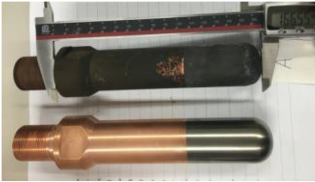
FIG. 9. Macromorphology of the contact surface.
