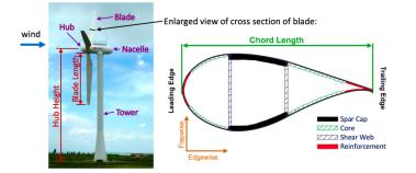
Figure 2: The major components of an (upwind) wind turbine (left) and of each blade (right). The wind turbine rotor consists of the hub and the blades. [Left photo courtesy of L. Fingersh.]
