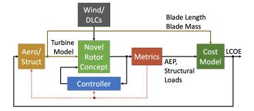
Figure 5: Block diagram illustrating our integrated wind turbine design process, which we applied in multiple design iterations on the novel SUMR concept to reduce the LCOE relative to the CONR-13.
