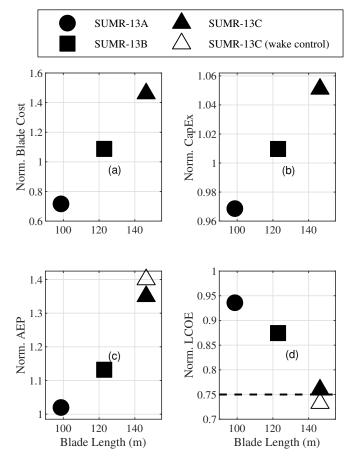
Figure 12: These plots show the impact of blade length for a 13 MW two-bladed downwind rotor relative to a conventional upwind 3bladed rotor on (a) blade cost, (b) capital expenditures (CapEx), (c) annual energy produced (AEP), and (d) levelized cost of energy (LCOE). All results are normalized relative to the CONR-13. Additional wind farm wake control effects were explored for the SUMR-13C, where further benefits in AEP and LCOE can be achieved with downwind turbines.
