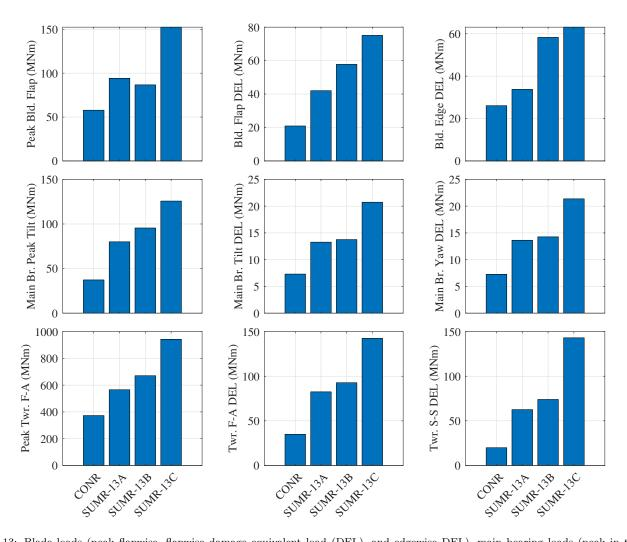
Figure 13: Blade loads (peak flapwise, flapwise damage equivalent load (DEL), and edgewise DEL), main bearing loads (peak in the tilt direction and DELs in the tilt and yaw directions), and tower loads (peak fore-aft (F-A), and DELs in the F-A and side-to-side (S-S) directions for the CONR-13, SUMR-13A, SUMR-13B, and SUMR-13C.
