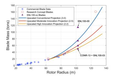
Figure 3: Blade mass trends with rotor size. The rotor radius is defined as the distance from the hub center to the end of the blade tip.
