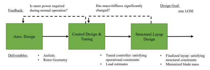
Figure 8: A single rotor design iteration, detailing the coordination among the aerodynamics, controls, and structures teams.
