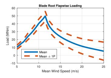
Figure 9: An example of the mean and 1P load component of the blade flapwise load of the SUMR-13A, which was used to estimate the peak and fatigue loading of the rotor.
