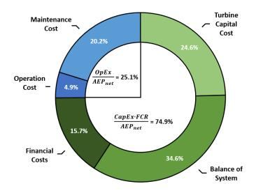
Figure 7: Breakdown of Capital Expenditures (CapEx) and Operational Expenditures (OpEx) as a percentage of Levelized Cost of Energy (LCOE) for offshore, fixed-bottom wind plants based on data from [2].
