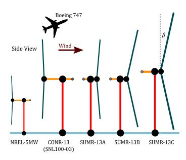
Figure 6: Diagrams of the turbines designed and analyzed in this study, along with the NREL-5MW reference turbine [25] for comparison. Tower heights, rotor radii, and cone angles ( $\beta$ ) are drawn to scale; overhangs and nacelle center-of-masses are enlarged for comparison.
