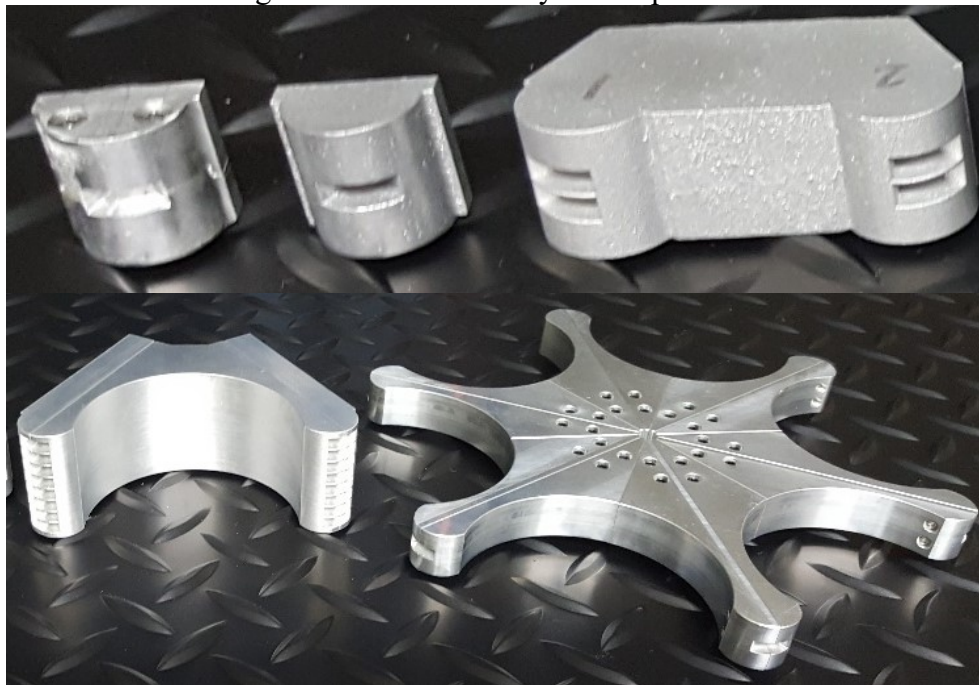
Fig. 3.1. Family of demonstrated curved aperture horn antennas. Left to right from top: single element (CNC and DMLS), 2 element array (DMLS), 8 element array (CNC) and circular array (CNC) configurations.
