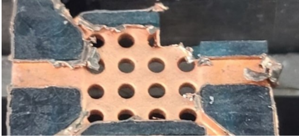
Fig. 6.15. Interior view of SLA coated piece after destructive test.
