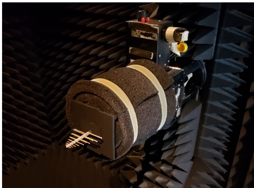
Fig 5.15. LPDA mounted in anechoic chamber.
