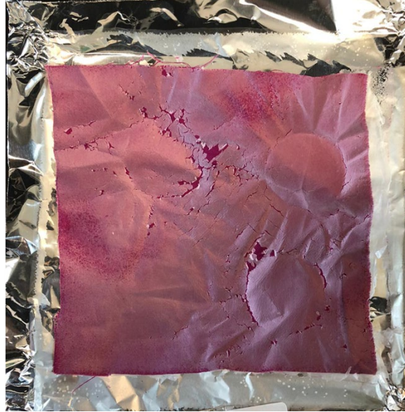
Figure 23. CNF coated sample fabric with visible cracks after it was removed from the funnel.
