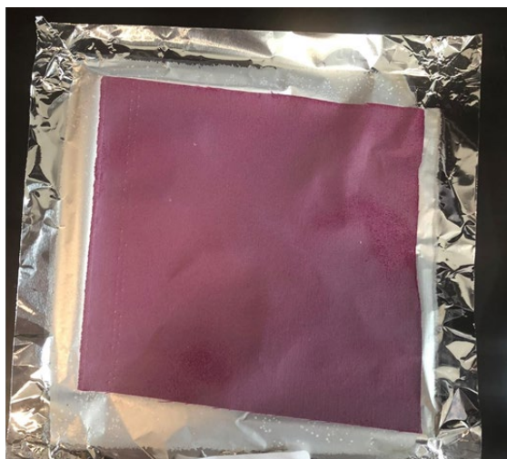
Figure 21. Oven dried CNF coated sample fabric.
