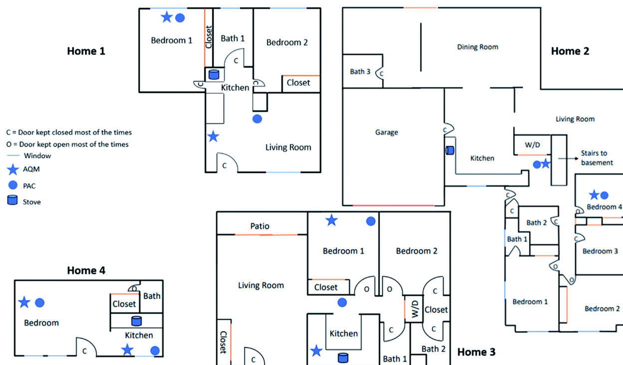
Figure 1. Layouts for all the locations used for this study. Note all the layouts are approximate to scale (1":16' for a printed page). The OPS and AQMs were placed on a wire shelf rack, at either 0.3 m or 0.6 m above the floor.
