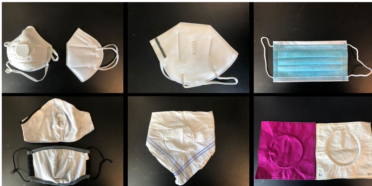
Figure C1. Different samples that were used in this study are shown from top right to bottom in clockwise direction: N95 respirator, KN95 respirator, Surgical mask (SM), wash/dry sample coupon, 2-ply bandana and Cloth mask (CM).
