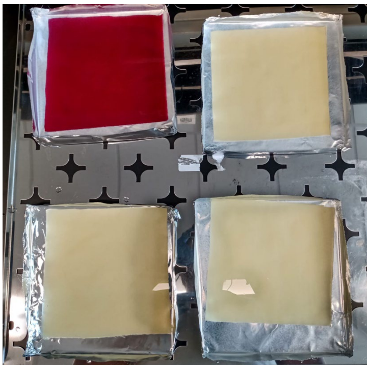
Figure 20. Fabric samples soaked in CNF suspension before drying.
