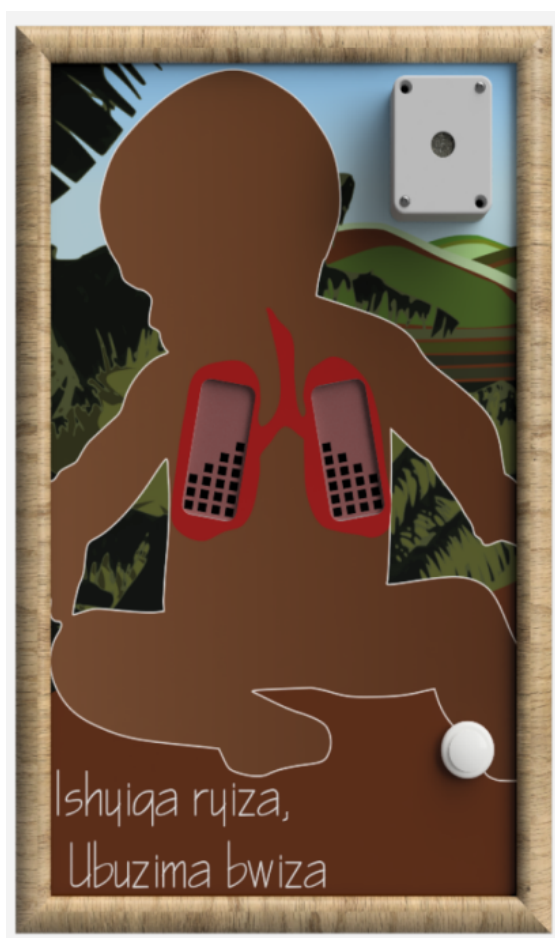
Figure 2. The air quality monitor and feedback device. The device includes an air quality sensor ( top right ), a clean cooking message in the participants' first language ( bottom left ), a display of real-time air quality data, and a built-in sound system for sudden air quality change alarm.
