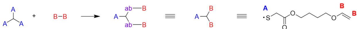
Figure 3.10: Schematic representation of the disulfide-ene reaction of DSDVE. This representation is a depiction of the fundamental reactive unit obtained after radical cleavage of the disulfide. ‘A’ depicts a thiyl radical and the ‘B’ represent the alkene that acts as a difunctional unit.
