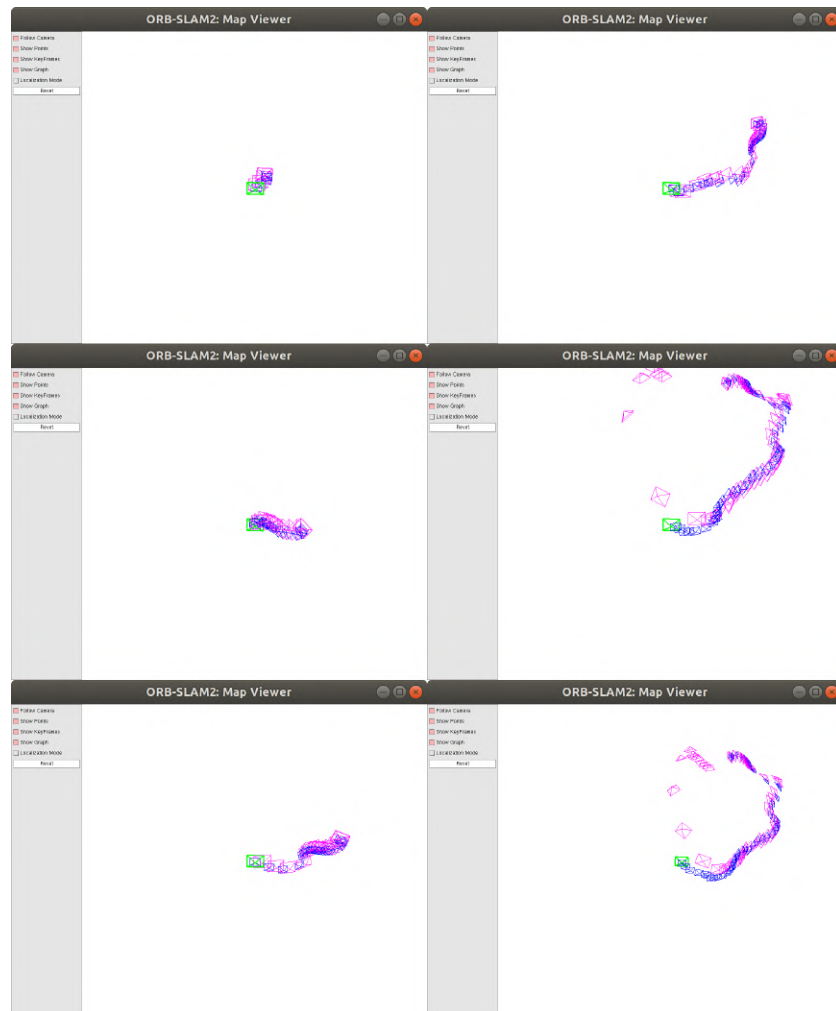
Figure 2.5: TUM RGB-D fr1-desk dataset tracking result. The pink frames are from the direct method, while the blue frames are from the ORBSLAM. There is a rapid turn in the TUM RGB-D fr1-desk dataset, which leads to failure tracking. See the right column
