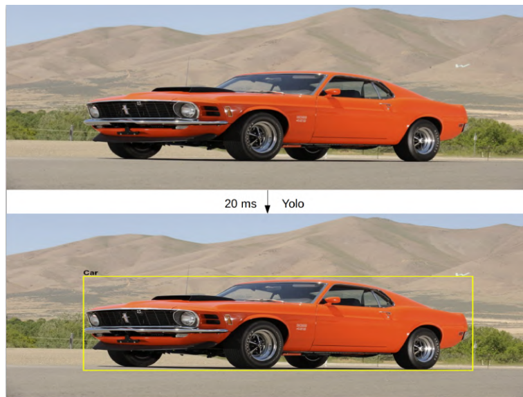
Figure 1.2: Image object detector Yolo. In 2015 it can use GPU Titan X achieves realtime object detection.
