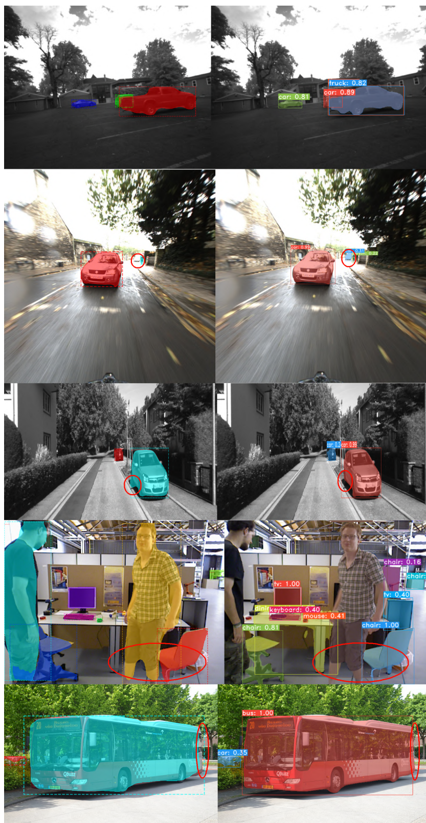
Figure 3.12: The left side is the detection from the MaskRCNN, and the right side is the detection from Yolact. The red circles show the Yolact has better mask quality than the Mask RCNN. The Yolact misses a person detection in the fourth image. The phenomenon can be relieved by decreasing the detection threshold.
