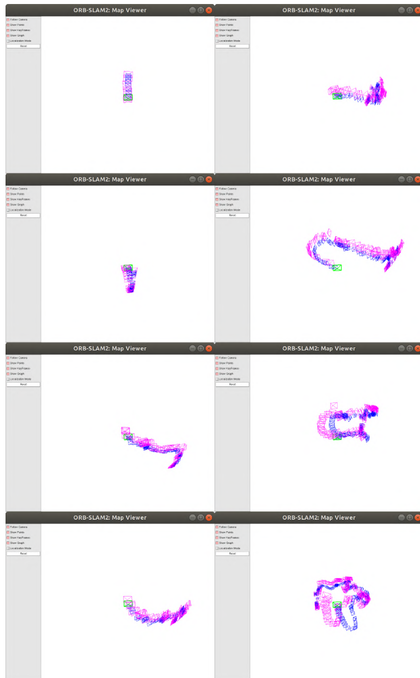
Figure 2.4: TUM RGB-D fr1-teddy dataset tracking result. The blue frames result from the original ORBSLAM, and the pink frames result from the direct method. The direct method follows the ORBSLAM initially but has a more considerable drift as we have more and more frames.
