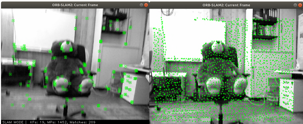
Figure 2.3: The left side of the image shows the result of the original ORBSLAM2 feature. The right side of the image shows the effect of high gradient pixels. i.e. “direct features”. The ORB features are more sparse than the direct features. Instead of choosing features with gradients larger than a threshold, we choose features in each 7 by 7 or 9 by 9 pattern. In this way, the high gradient pixels spread out to the whole image.
