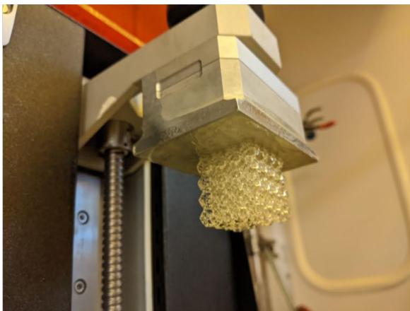
Figure 4.11 a) Top-down platform for stereolithography (SLA) 3D printing. b) Sample print of a 27 x 27 x 27 mm 3 lattice cube based on triazole/thiol-norbornene photopolymerization.
