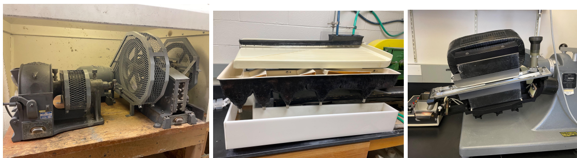
Figure 5: Mineral separation techniques including crusher/grinder (left), water table (center), and magnetic separator (right).
