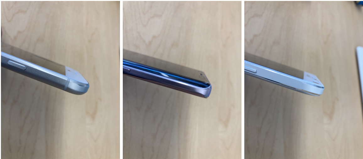
Figure 8.1: Different materials for frame body: Pixel XL(Aluminum), Galaxy Note9(Aluminum), Galaxy Note4(Plastic).
