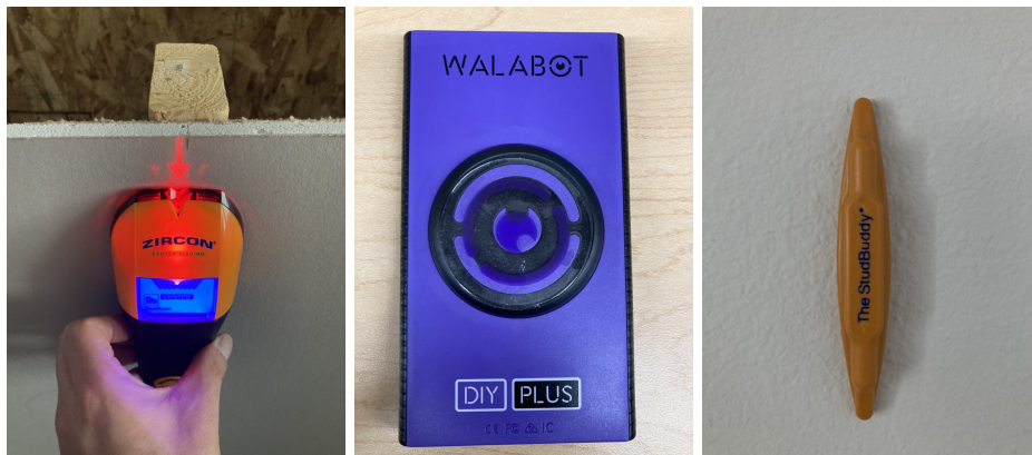
Figure 7.1: Stud finders used for finding a ground-truth location of a stud: electronic stud finder (HD70), radar stud finder (Walabot), and magnetic stud finder (StudBuddy).
