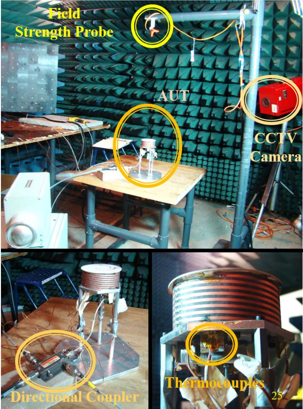
Figure B.2: Measurement setup for the high power test of the 94 mm diameter aperture planar spiral-helix antenna.
