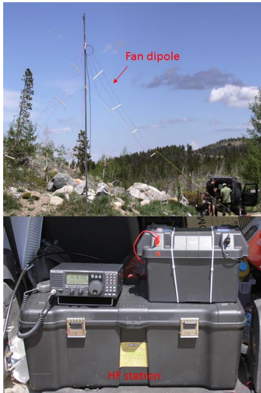
Figure 3.12: Setup for the HF station at the remote site for the preliminary testing of the two arms half-loop antenna at the University of Colorado Boulder.
