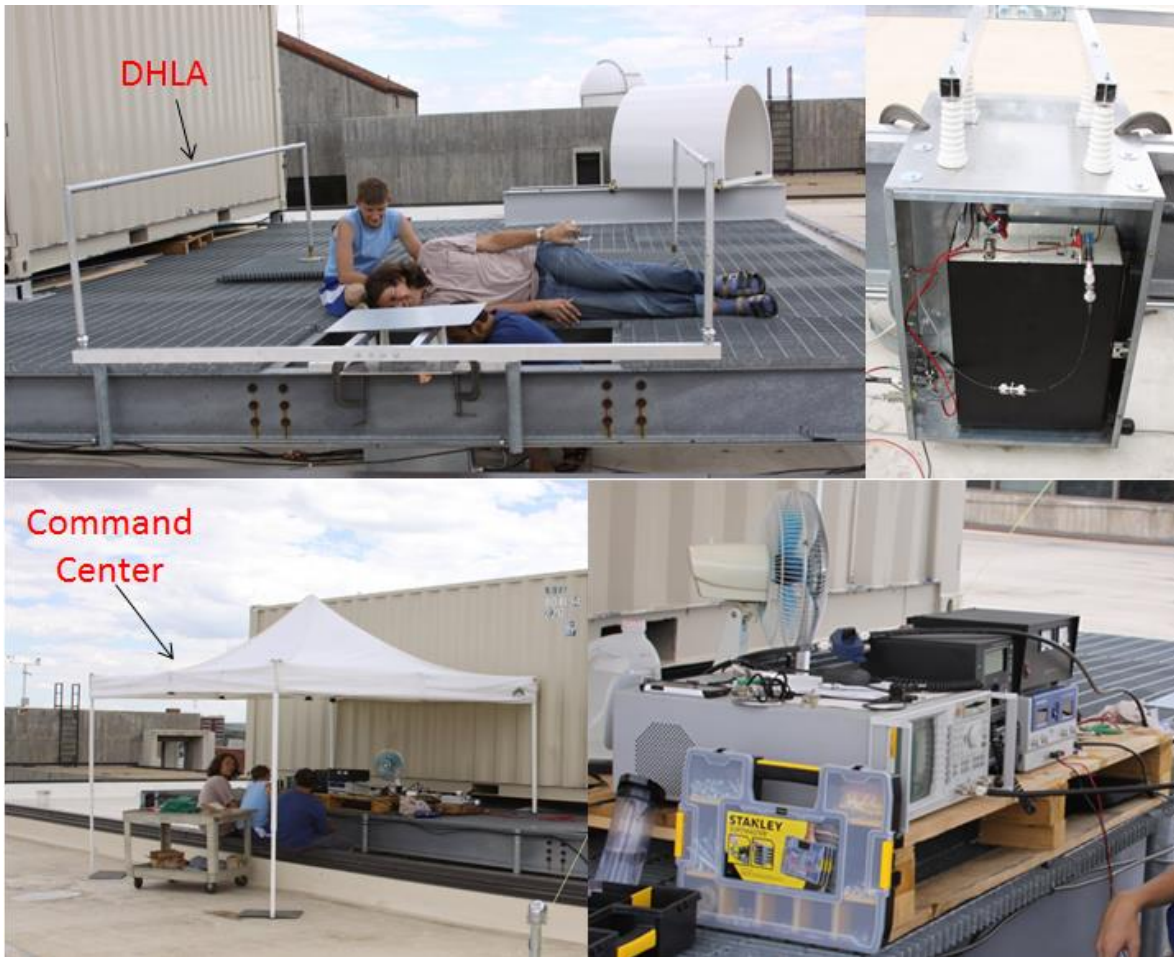
Figure 3.11: Setup for the HF station atop the roof of the engineering center at the University of Colorado Boulder. Seen in the top inset is the structure of the antenna configures in the Dual Arm Half Loop Antenna (DHHLA) mode. The top right inset shows the details of the tuner box, the feed region and the COTS tuner installed inside the tuner box [34].
