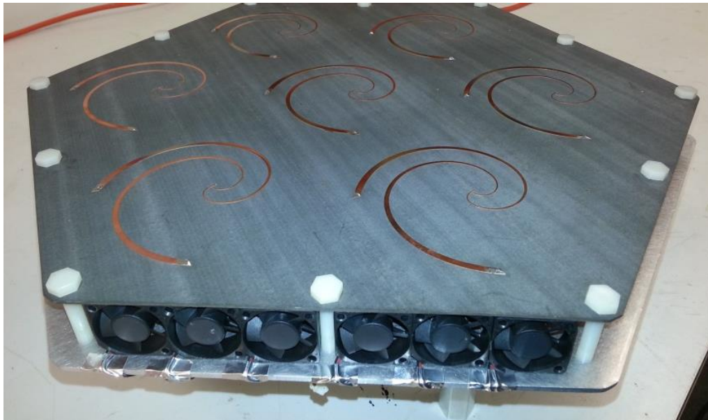
Figure B.11: Resistively-loaded, FI array made from spiral antenna elements with active cooling fans mounted on the antenna sidewalls.
