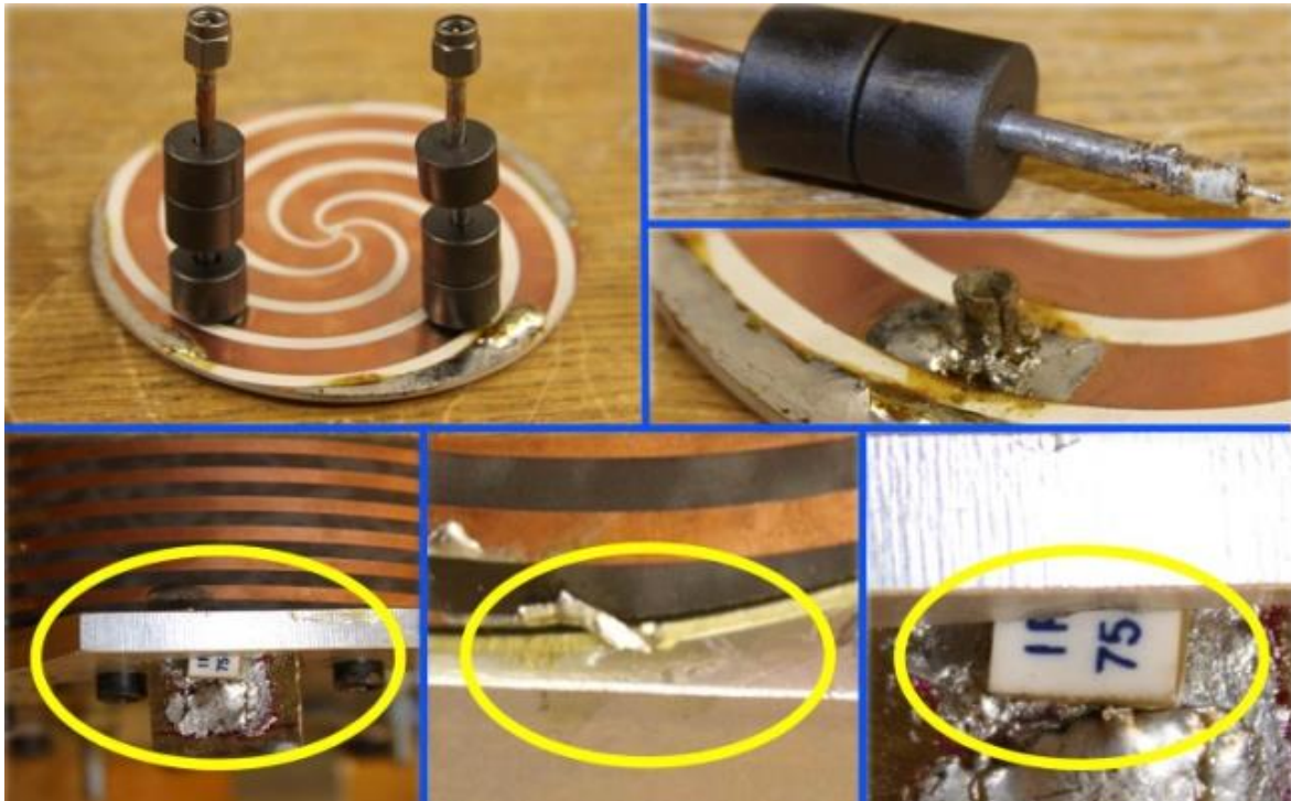
Figure B.6: Spiral helix antenna dismantled after the high-power test as part of the antenna autopsy investigation. Contribution from each part of the antenna led to the catastrophic failure of the antenna during the high- power tests.
