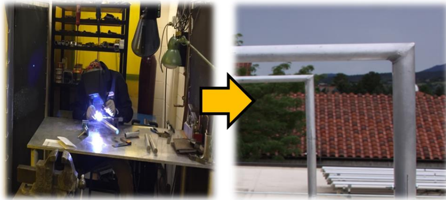
Welding the right angle sections of the antenna
