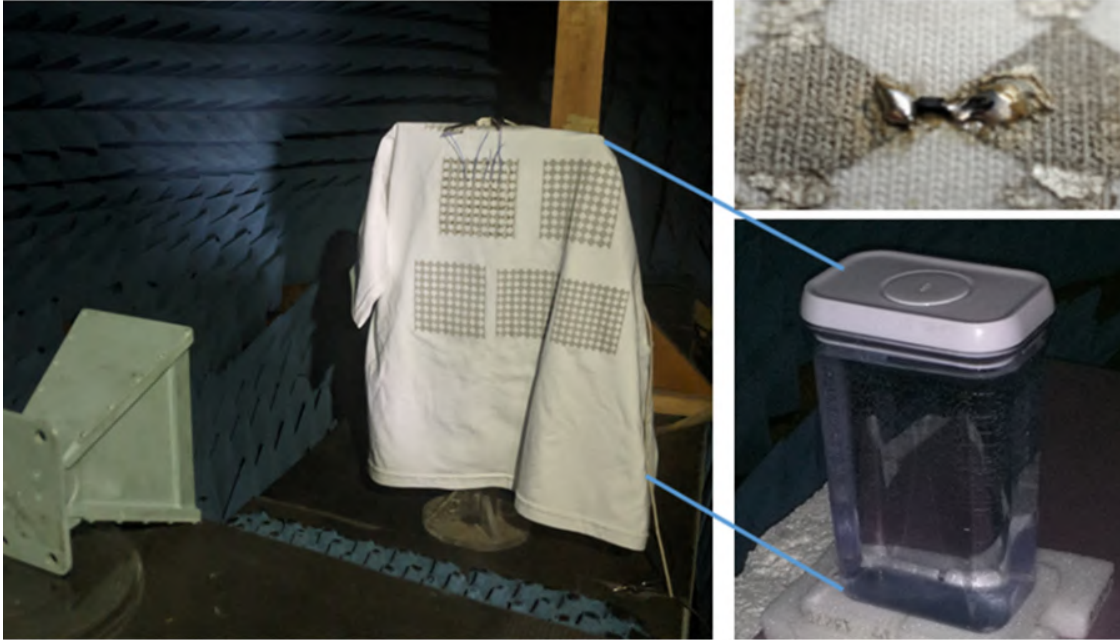
Figure 9.19: Photo of tee-shirt on phantom in the anechoic chamber during measurements, with the phantom shown on the bottom right. A detail of a fabricated single array element is shown on the upper right.
