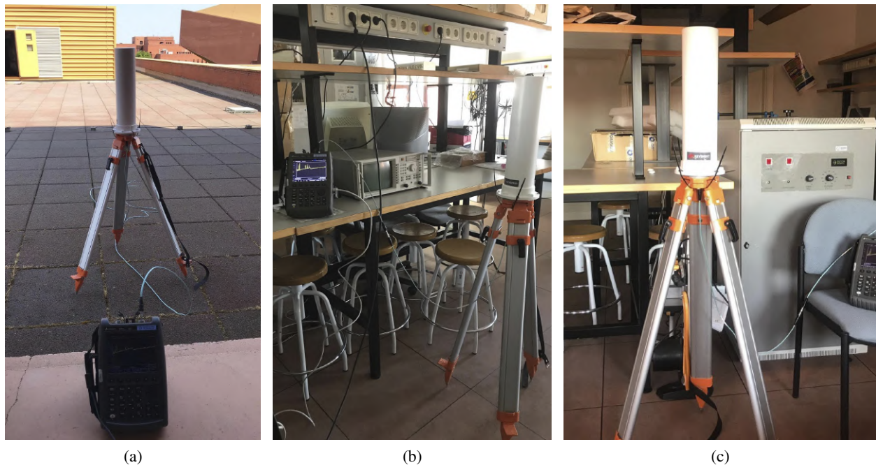
Figure 9.2: Ambient RF spectrum monitoring locations for three different scenarios: (a) roof, (b) laboratory 1 and (c) laboratory 2. Measurements were performed using a calibrated Keysight N6850A broadband omnidirectional antenna and a N9918A FieldFox 26.5-GHz handheld microwave analyzer.
