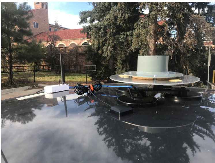
Figure 2.3: Receiver system: omni directional antenna and RTK GPS rover station mounted on a car roof
