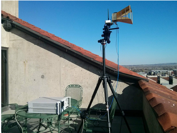
Figure 2.2: TX system: signal generator, horn antenna and RTK GPS base station
