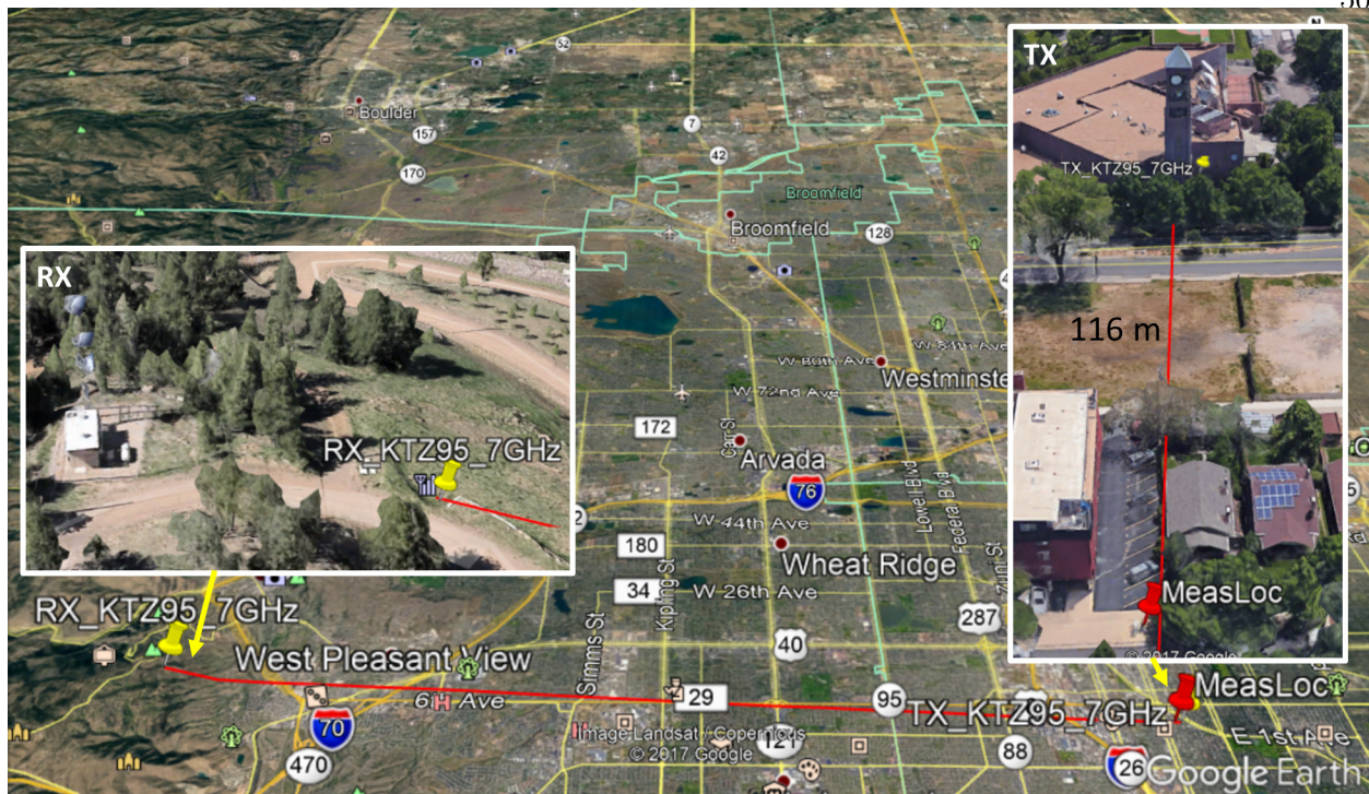
Figure 3.6: BAS fixed link and measurement location.
