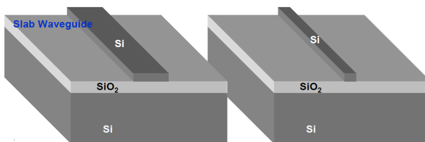
Figure 2.5: We can approximate the modes in x direction as a slab waveguide for the left structure. However we can not compute the y direction modes using the slab waveguide approximation. The right structure is the one we will be dealing with for our designs. It can have air cladding or SiO_2 cladding.
