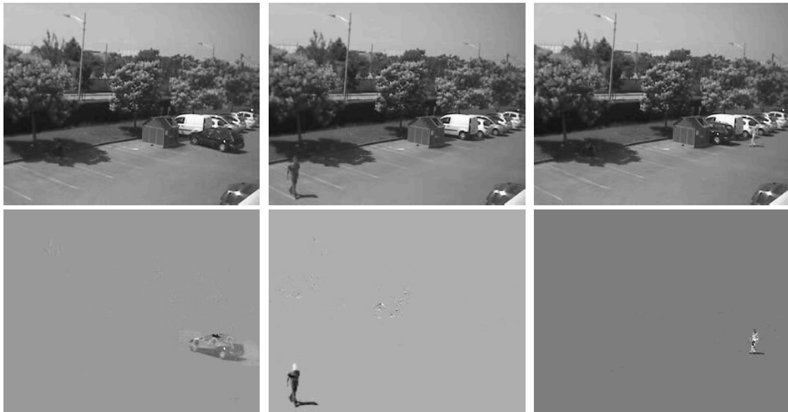
Figure 10: Real-time background subtraction using Split-SPCP. Split-SPCP correctly identifies (left) a car in the middle-ground, (center) a person in the foreground, and (right) a person in the background. The resolution is 240 \times 320 pixels per frame, 600 frames were decomposed at one time, and only 200 iterations were allowed.
