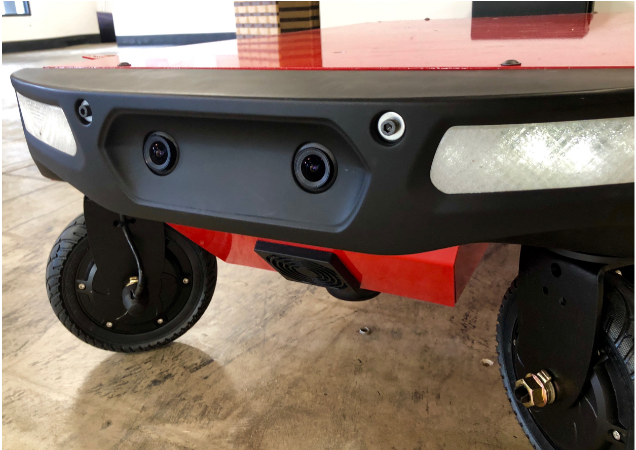
Figure 7.1: Robotic platform equipped with two camera stereo pairs, one in front and one in the back, used for experiments.
