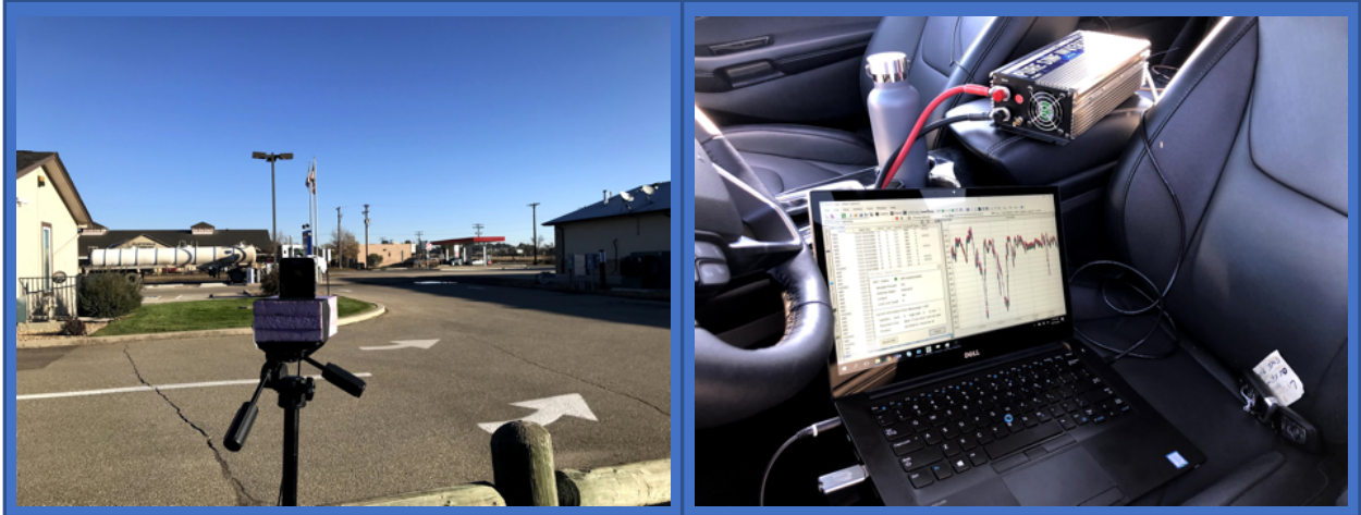
Figure 9, The data collection setup for a stationary data collection of an eNB output power.
