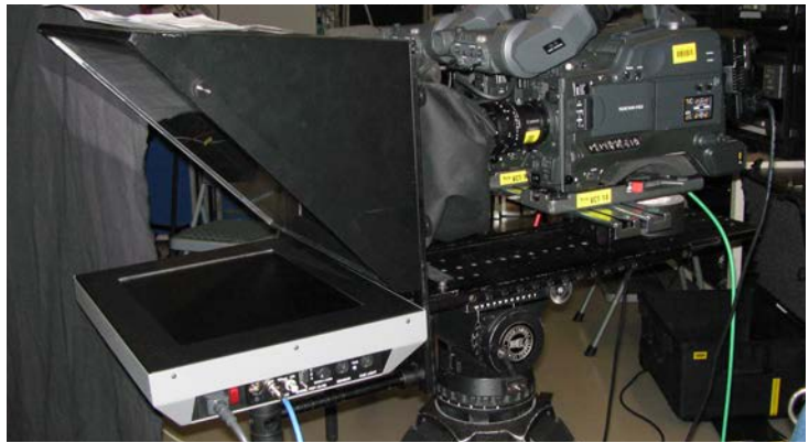
Two camcorders behind a single teleprompter glass allowed us to shoot two framings at the same time for each interview
