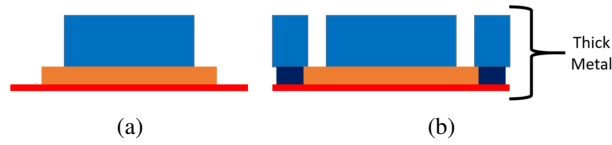
Figure 3.3: Standard broadside-coupled transformer cross-section (a) and modified transformer cross-section (b).
