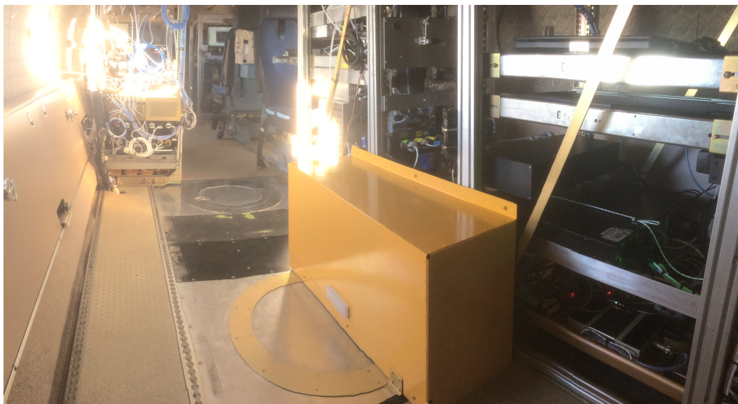
Figure 6.2: View of the mounted POLAR sensor in the GV cabin. The acquisition unit, detector controllers, and laser controller are shown on the lowest tray of the right hand side rack. The top tray has the acquisition computer to manage data collection, accessed remotely from aircraft's rear.
