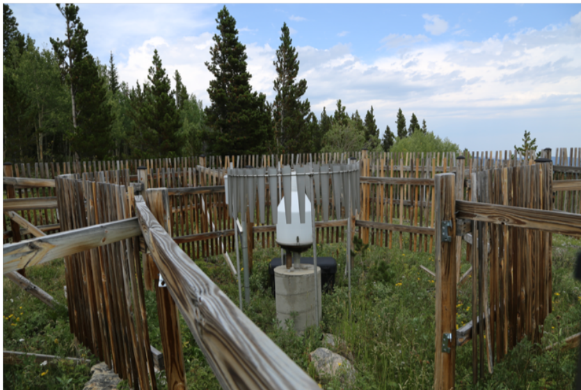
Figure 2-11: USCRN sDFIR near the C1 site. Geonor gauge is in the center and immediately surrounded by the single Alter Shield. The two concentric and hexagonal wind fences are also shown.
