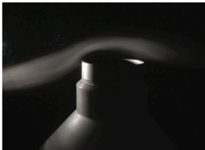
Figure 1-1: Airflow around the orifice of a standard precipitation gauge as mapped with laminar wind tunnel flow (Rasmussen et al. 2012).
