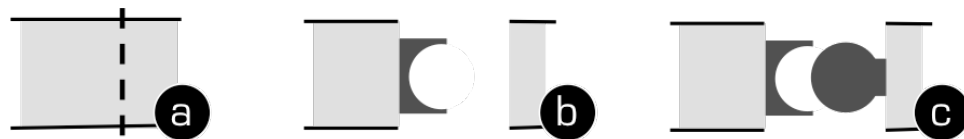
Figure 4.2.10: Operations to insert a modular ball joint in a model: (a) Slice the model in two; (b) subtract space to create room for the joint and add the female connector; (c) add the male part.
